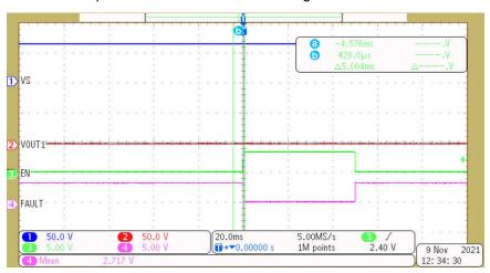
Figure 3-2. Over-Voltage Protection with the Switch Toggling at 60 V
