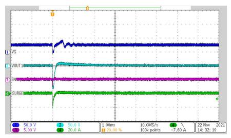
Figure 4-9. Waveform with Negative Surge Applied at VOUT and EN is Low
