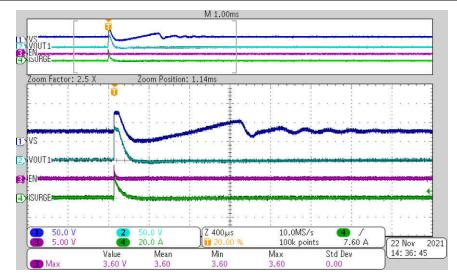
Figure 4-8. Waveform with Positive Surge Applied at VOUT and EN is Low
