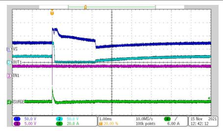
Figure 4-4. Waveform with Positive Surge Applied on VS
