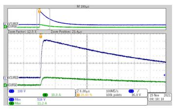
Figure 4-1. Surge Waveform on Resistive Load
