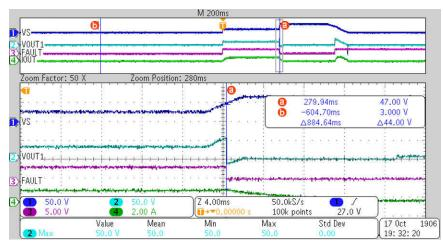
Figure 3-1. Over-Voltage Protection During ON State with Supply Ramping
