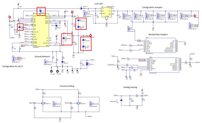
Figure 2-1. TPS272C45C Schematics for 60-V Tolerance
