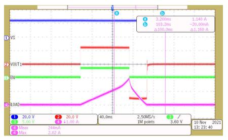
Figure 5-2. Waveform for the Inductive Switching Transition at 2 A Turn-off Current
