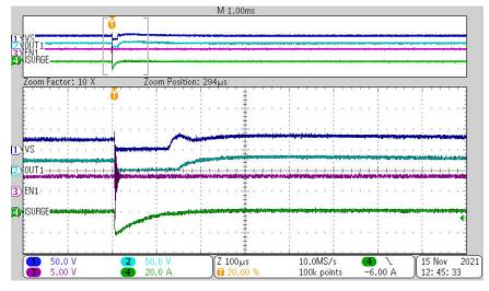
Figure 4-5. Waveform with Negative Surge Applied at VS
