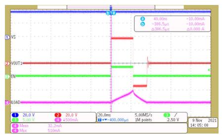
Figure 5-1. Waveform for the Inductive Switching Transition at 500 mA Turn-off Current
