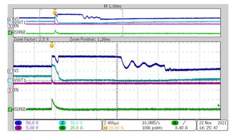
Figure 4-6. Waveform with Positive Surge Applied at VOUT and EN is High
