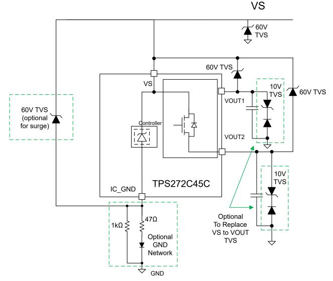
Figure 2-2. Simplified Diagram for the Main Components Needed for 60-V Tolerance
