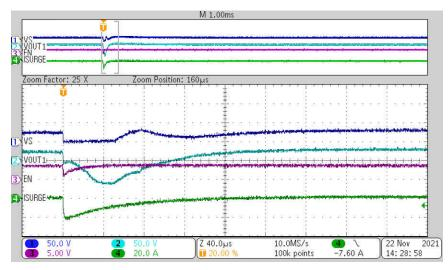
Figure 4-7. Waveform with Negative Surge Applied at VOUT and EN is High
