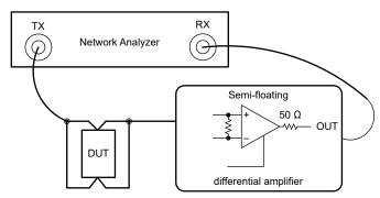
Figure 2-2. 2-Port Shunt-Through Circuit Configuration
