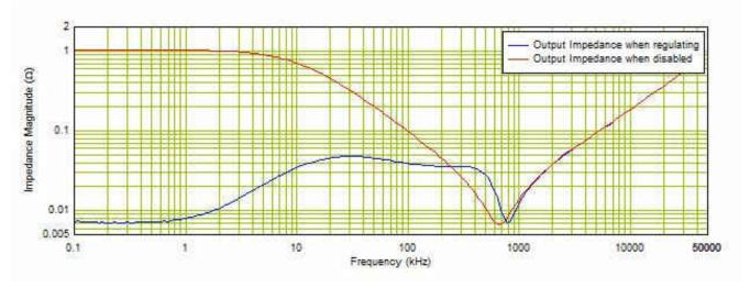
Figure 5-1. Output Impedance Measurements of the TPS62A01 Connected to a Resistive Load
