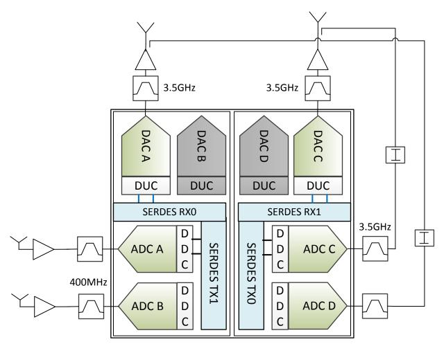
Figure 12. 2T2R2FB Configuration for RF Repeater
