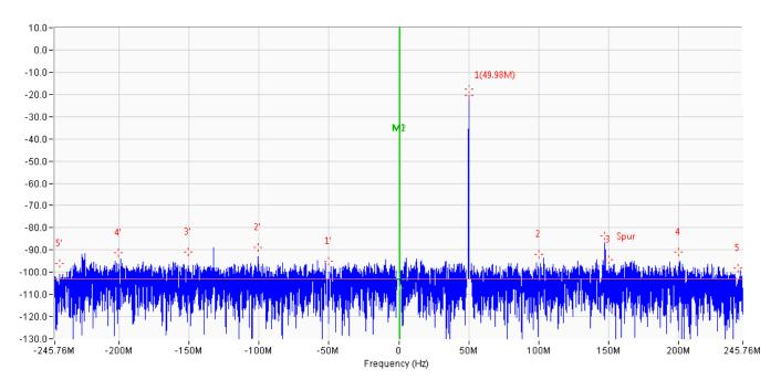
Figure 14. FBRX Path Output with Single Tone at 1750MHz, -15dBFs
