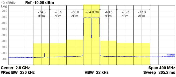
Figure 15. TX Output : 2x20MHz LTE Signal at 2.6GHz
