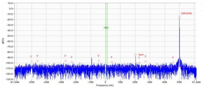
Figure 13. RX Path Output with Single Tone at 1750MHz, -15dBFS
