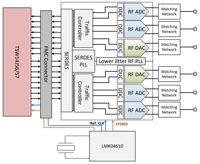
Figure 3. TSW0486 EVM Test Setup
