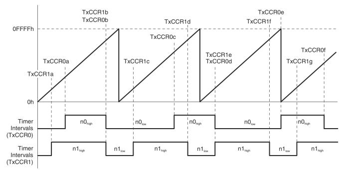
Figure 3-1. Continuous Mode PWM Generation
