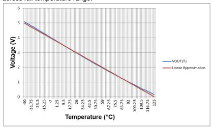
8. Solving the resistor network for the optimized temperature range improved the accuracy across the overall temperature range of the sensor. The temperature error across the optimized temperature range is approximately 1.65°C which occurs at 49.1°C. The temperature reading from the ADC is approximately 50.75°C while the actual temperature is 49.1°C. However, the error at the end points increases.
