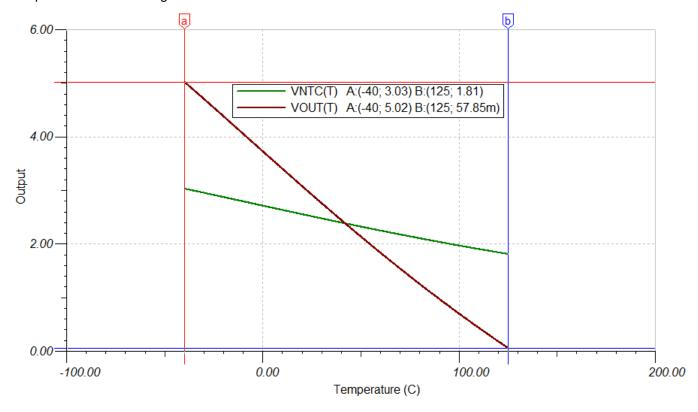
The output voltage curve is not linear and appears almost quadratic. This is due to the TMP61 thermistor response across temperature and the inherent non-linearity of a voltage divider.
