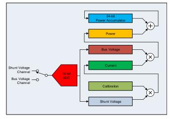
Figure 2. INA233 Power Conversion Engine
