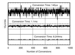
Figure 3. Noise vs. ADC Conversion Time
