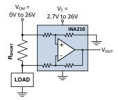
Figure 2. INA210: Current Sensing Amplifier
