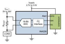
Figure 3. Digital Current/Power Monitor
