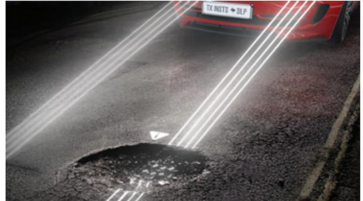
**Figure 6.** DLP headlights working with the ADAS camera systems to detect and alert drivers to objects in the road.
