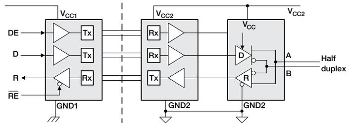
**Figure 4.** A functional diagram of the ISO1500 isolated RS-485 transceiver containing an integrated galvanic isolation barrier in a 4.90-mm  $\times$  3.9-mm 16-pin shrink small-outline package (SS016).
