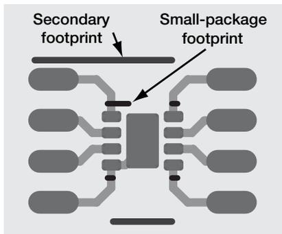
**Figure 5.** Second-source solution example for PCB layout.
