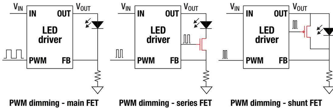
Figure 10. LED illumination PWM dimming methods.
