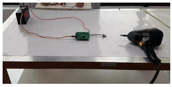
Figure 37. IEC61000-4-2 ESD Test Setup for TIDA-010046
