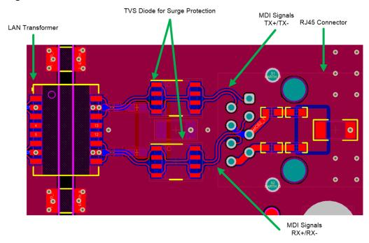
Figure 19. MDI Connections Between Isolation Transformer and RJ45 Connector
