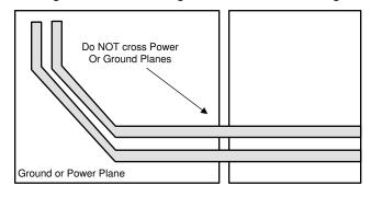
Figure 18. Differential Signal Traces
