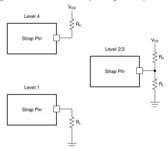
Figure 3. Four-Level Bootstrap Configuration (DP83822I)
