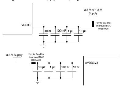
Figure 10. Power Supply Decoupling Recommendation
