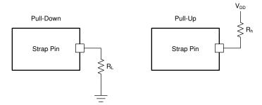
All the strap pins have the provision for populating the strap resistors for Ethernet PHYs on both PSE and PD side boards to place the device in to a specific configuration as desired.
