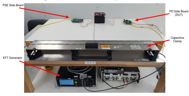
Figure 38. IEC61000-4-4 EFT Test Setup for TIDA-010046
