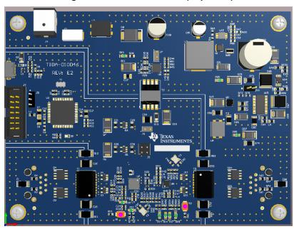
Figure 23. PSE Side Board (Top View)
