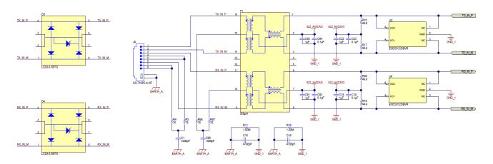
Figure 21. Recommended 10/100 Mbps Twisted Pair Interfaces and Bob Smith Termination for PoE Port as on PSE Side Board
