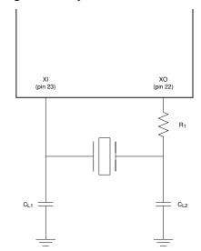
Figure 14. Crystal Oscillator Circuit
