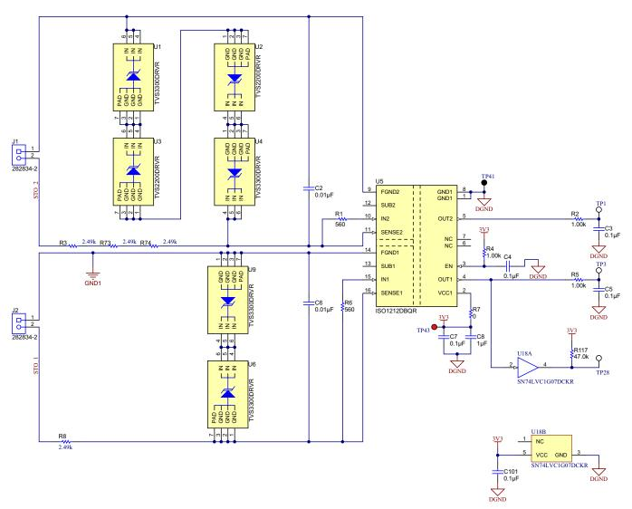
Figure 10. Isolated 24-V, 48-V Binary Input Receiver
