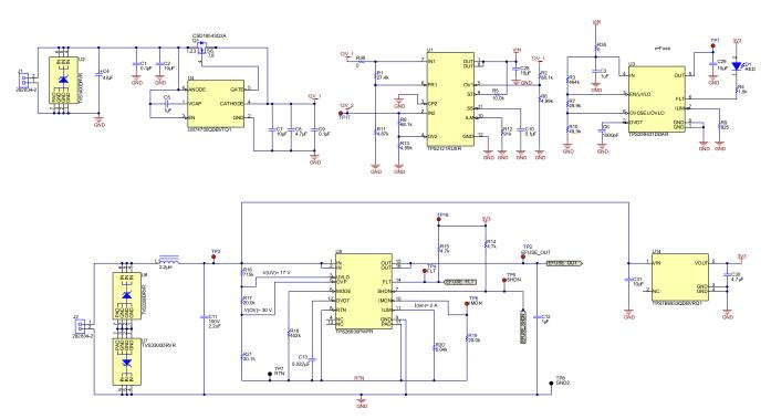
Figure 19. DC Input Protection for 12-V and 24-V Inputs
