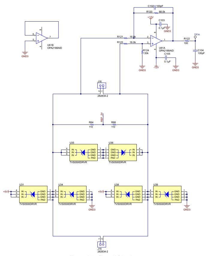
Figure 8. Delta-Sigma ADC Interface
