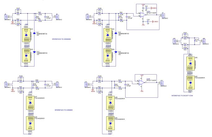
Figure 4. ADS8588S Interface Configuration Using Unidirectional TVS
