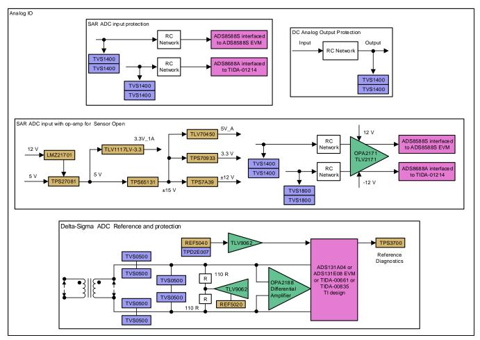
Figure 2. Power Analog IO
