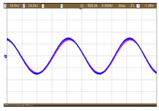
Figure 26. ADC Input With TVS Below Breakdown
