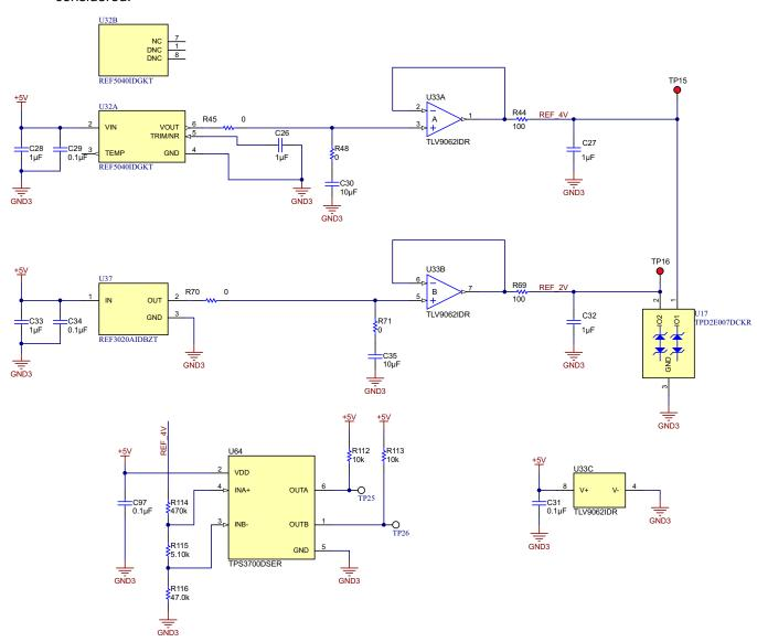
Figure 9. Delta-Sigma ADC Reference Buffer Protection
