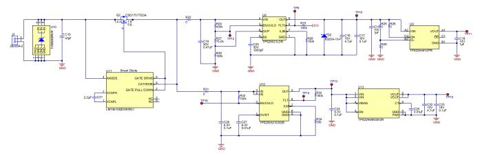
Figure 18. DC Input Protection for 5-V Input
