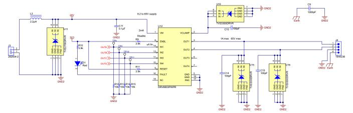
Figure 12. Low-Side Digital Output
