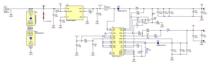
Figure 14. 5-V Dual-Output Supply
