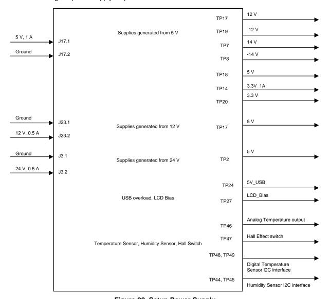
Figure 22. Setup Power Supply
