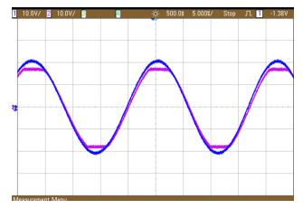
Figure 27. ADC Input With TVS1400 Breakdown
