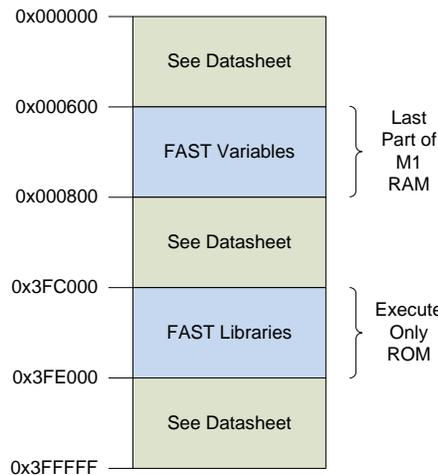
**Figure 7. 2802xF Allocated Memory for InstaSPIN-FOC Library**
