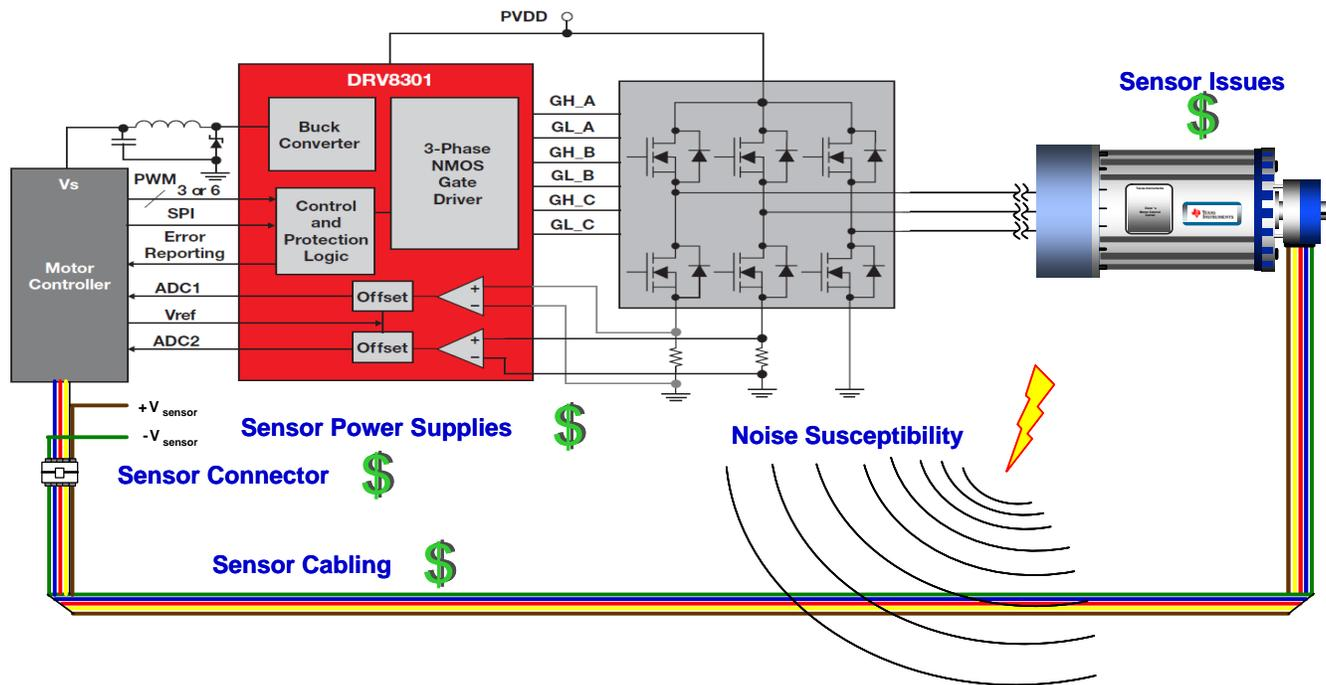
**Figure 3. Sensored FOC System**
