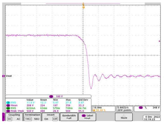
Figure 3-16. VDS, GaN Falling Edge Under 2.5-kW Load
