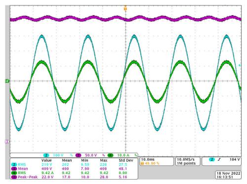
Figure 3-9. Waveform Under 220 VAC, 2 kW
