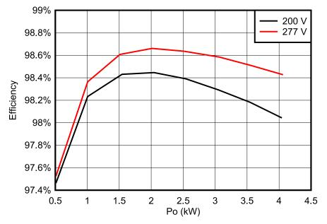
Figure 3-6. Efficiency Curve, 200 VAC and 277 VAC
