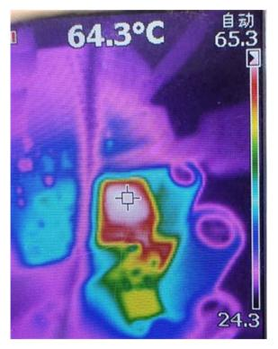
Figure 3-12. Temperature Rising of Buck Inductor L8
