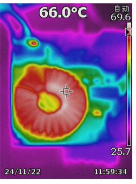
Figure 3-18. Boost Inductor Temperature
