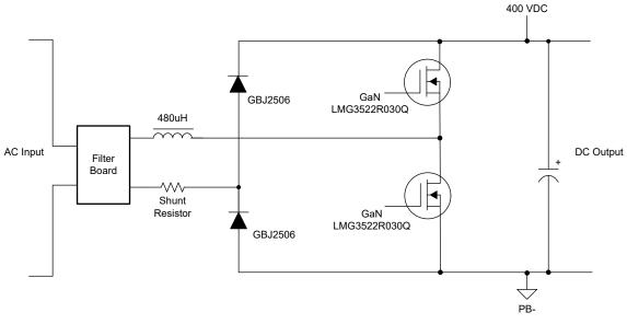
Figure 2-4. Power Stage Design Parameters
