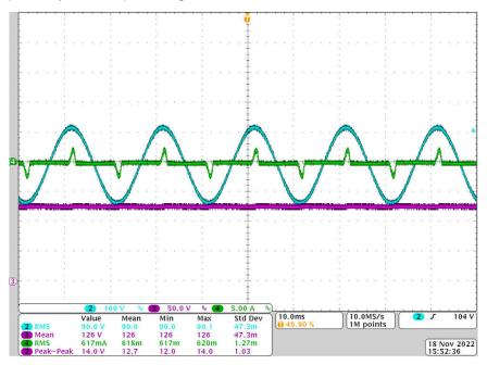
Figure 3-7. Waveform Under 90 VAC, 800- $\Omega$  Load
