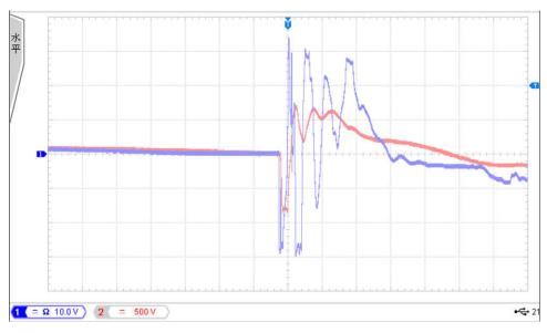
Figure 3-21. Surge Test Under 4 kV
