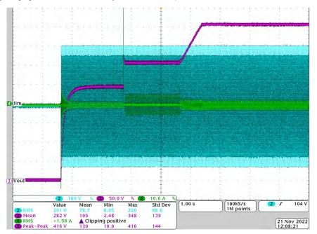
Figure 3-8. Power-On Sequence Under 220-VAC Input
