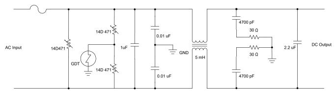
Figure 2-3. Filter Board Block Diagram
