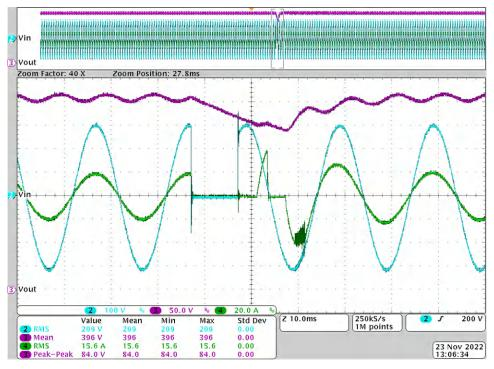
Figure 3-13. AC Drop at 90°, 10-ms Duration
