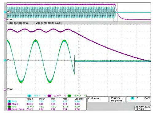
Figure 3-20. Power-Off Waveform
