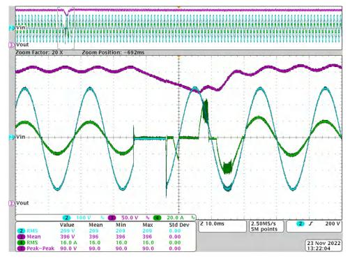
Figure 3-14. AC Drop at 45°, 10-ms Duration
