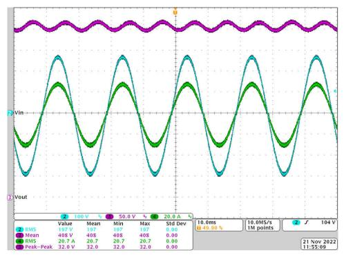
Figure 3-10. Waveform Under 220 VAC, 4 kW
