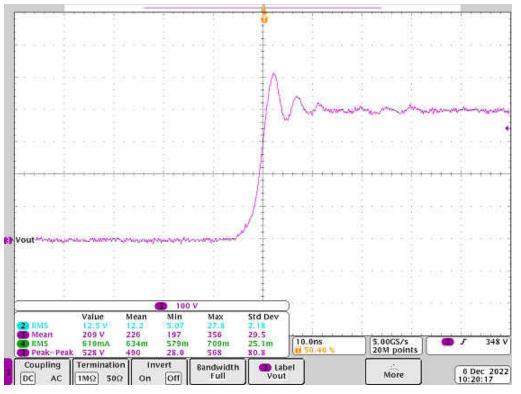
Figure 3-15. VDS, GaN Rising Edge Under 2.5-kW Load
