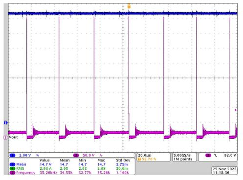
Figure 3-11. Buck Power-Supply Waveforms
