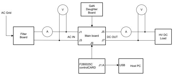
Figure 3-4. EUT Setup
