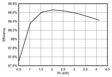
Figure 3-5. Efficiency Curve, 230 VAC
