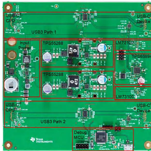
**Figure 2-2. PCB Subsection Overview**
