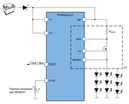
Figure 1. TIDA-01376 Block Diagram
