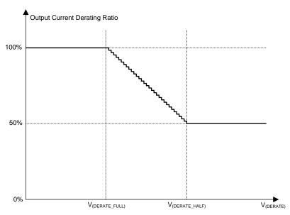
Figure 5. Output-Current Derating Profile
