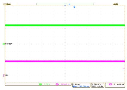
Figure 9. Operating Waveform,  $V_{IN}$  = 12 V CH3: Supply Voltage, CH4: Input Current
