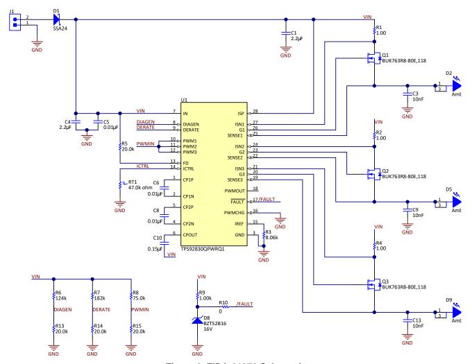
Figure 2. TIDA-01376 Schematic
