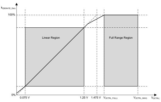
Figure 6. Analog Dimming Ratio
