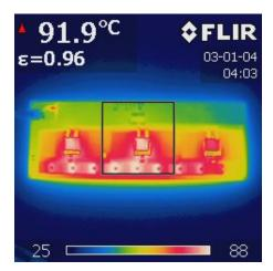
Figure 11. Thermal Image at 25°C, 12-V Input Voltage
