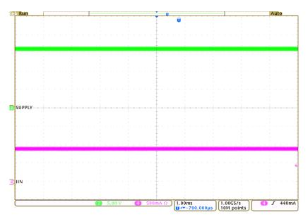
Figure 10. Operating Waveform,  $V_{IN}$  = 16 V CH3: Supply Voltage, CH4: Input Current
