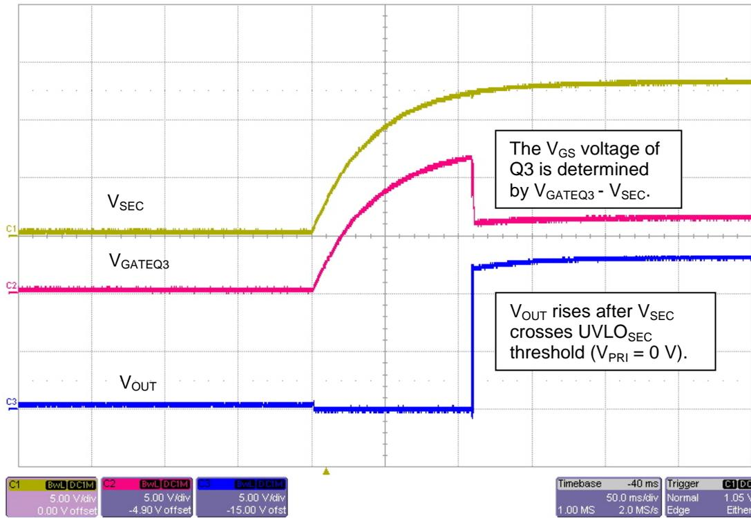
FIGURE 5:  $V_{SEC}$  Startup.  $V_{PRI} = 0$  V, Load = 65  $\Omega$
