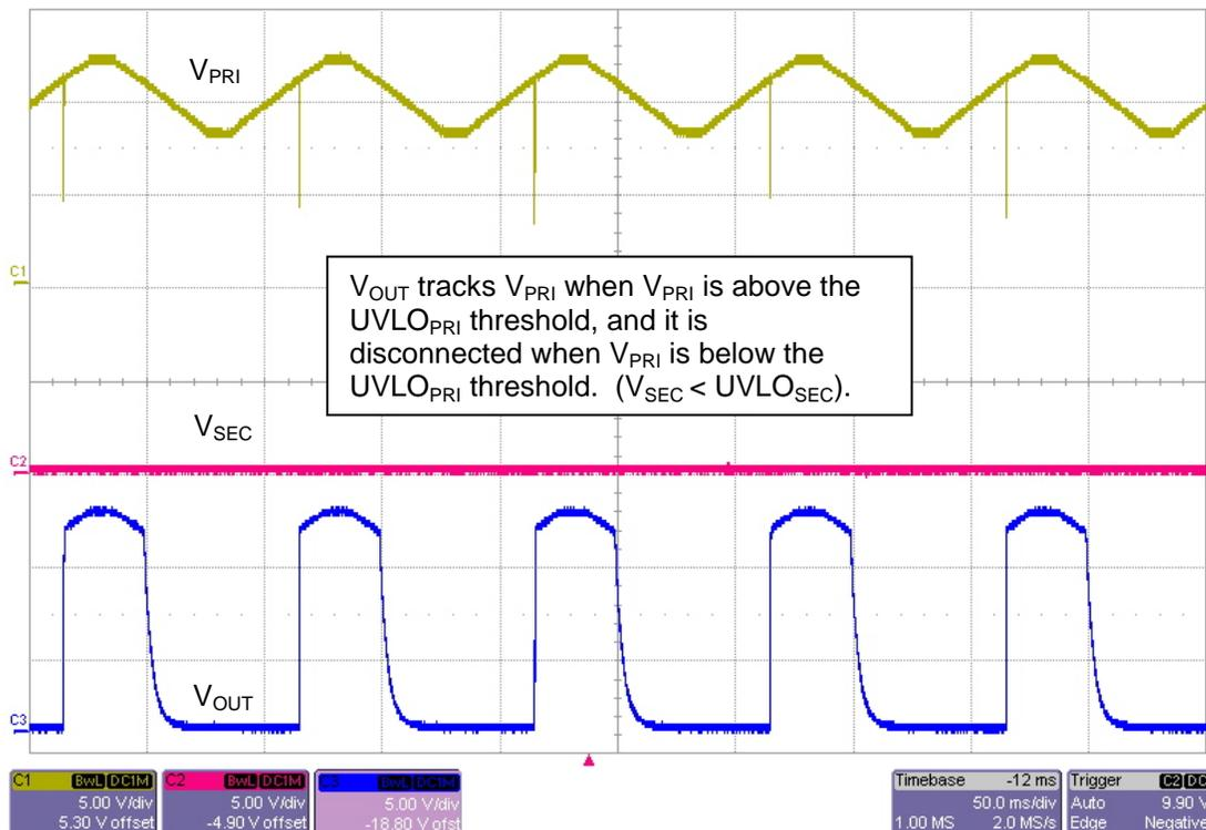
FIGURE 10:  $V_{PRI}$  Ramp.  $V_{SEC} = 0\text{ V}$ , Load =  $65\ \Omega$
