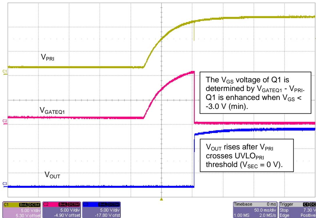
FIGURE 6:  $V_{PRI}$  Startup.  $V_{SEC} = 0$  V, Load = 65  $\Omega$
