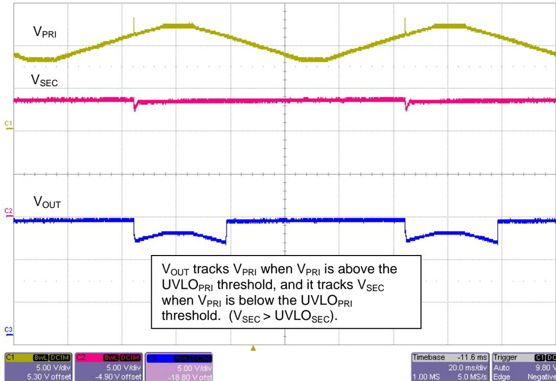
FIGURE 9:  $V_{PRI}$  Ramp.  $V_{SEC} = 13.5\text{ V}$ , Load =  $65\ \Omega$
