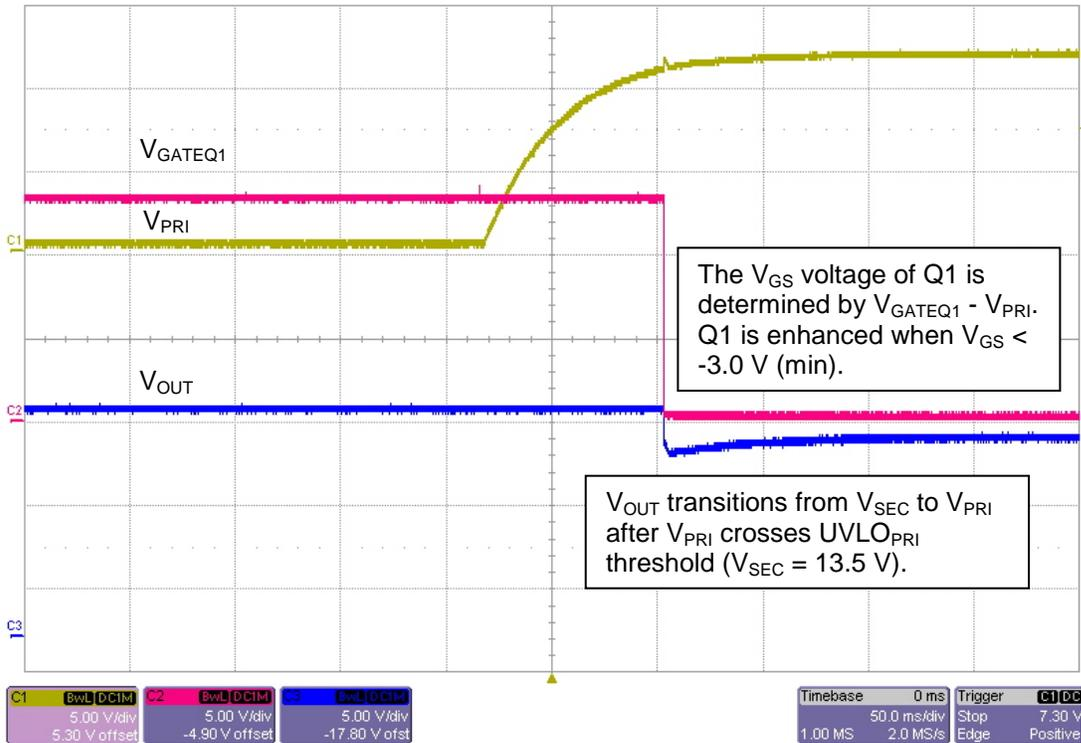
FIGURE 7:  $V_{PRI}$  Startup.  $V_{SEC} = 13.5$  V, Load = 65  $\Omega$
