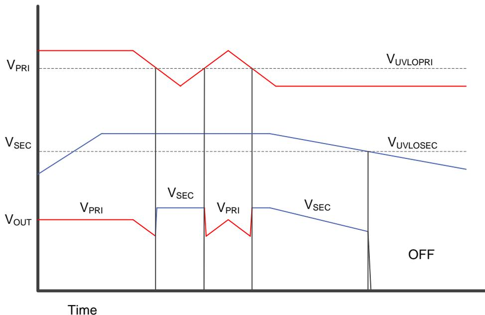
**Figure 3: Functional Timing Diagram**
