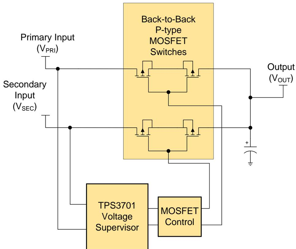
**Figure 2: Power Multiplexer Block Diagram**
