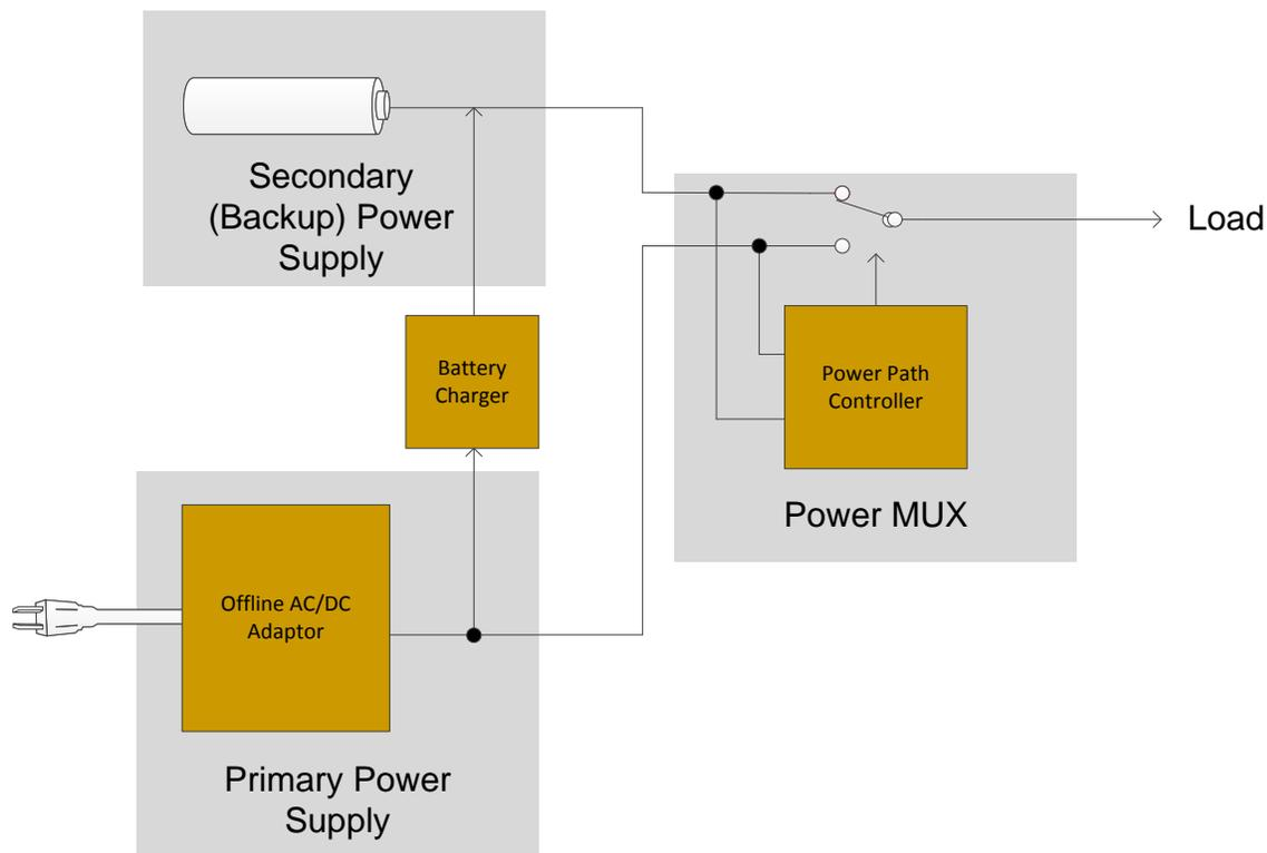
**Figure 1: Battery Backup Block Diagram**
