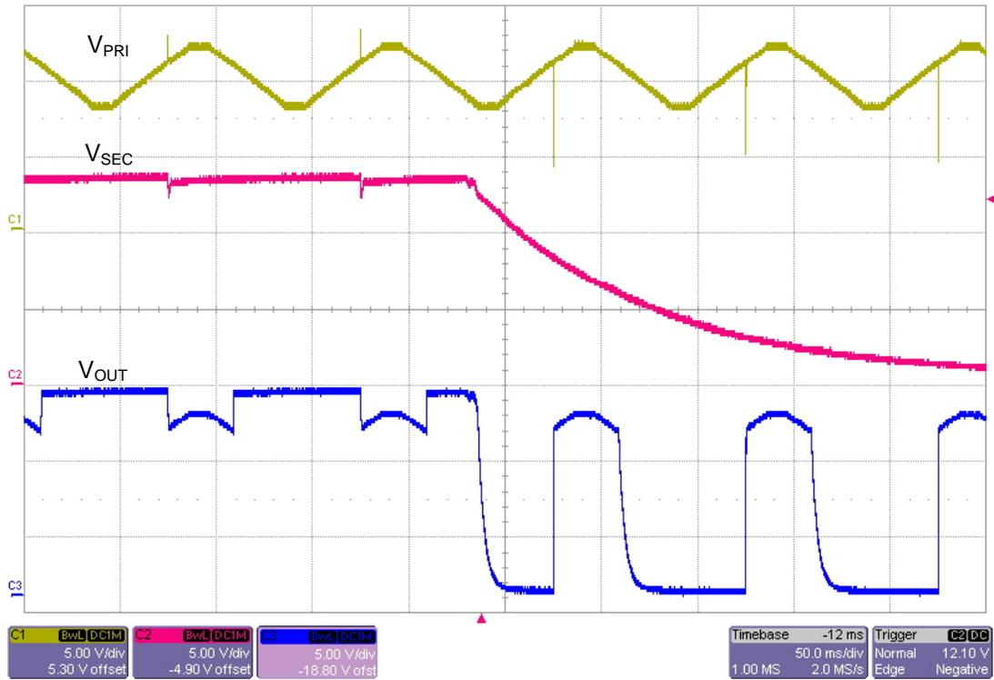
FIGURE 11:  $V_{PRI}$  Ramp.  $V_{SEC}$  = 13.5 to 0 V, Load = 65  $\Omega$
