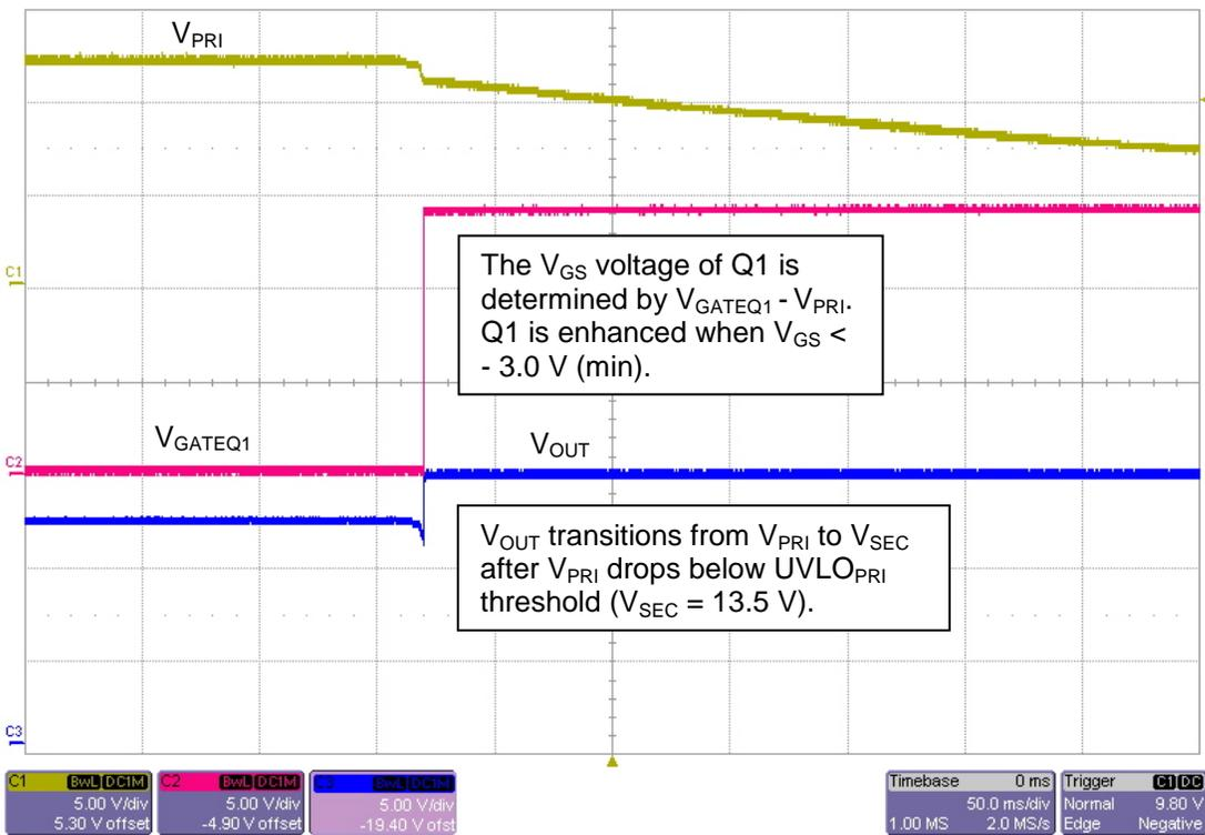
FIGURE 8:  $V_{PRI}$  Falling.  $V_{SEC} = 13.5$  V, Load = 65  $\Omega$
