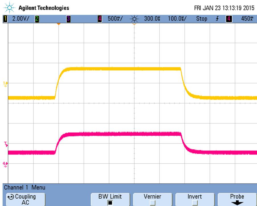
Figure 10 Output load transient at 24Vin, 4x LEDs
