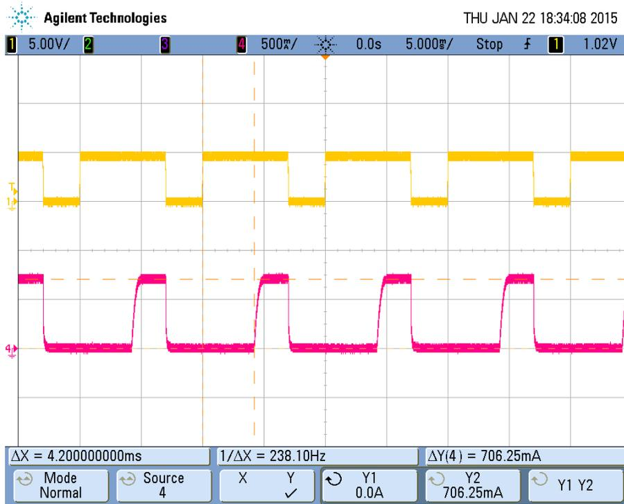
Figure 6 PWM at 70% duty cycle, average output current at 0.08A
