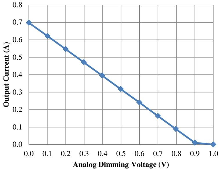
**Figure 5 Analog dimming voltage vs. output current**
