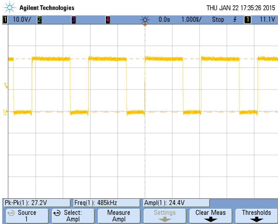
Figure 9 Switching waveform at 24Vin, 700mA, 4x LEDs
