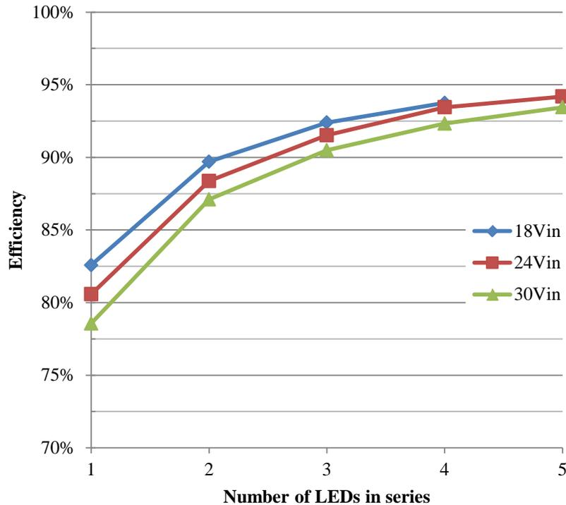
Figure 3 Power efficiency at 700mA output
