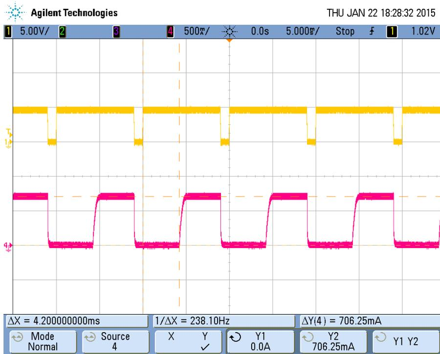
Figure 7 PWM at 90% duty cycle, average output current at 0.32A
