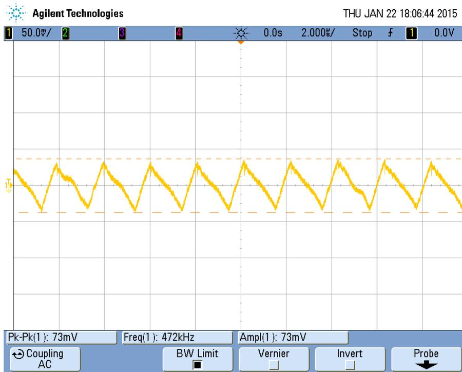
Figure 12 Input ripple at 24Vin, 700mA, 4x LEDs
