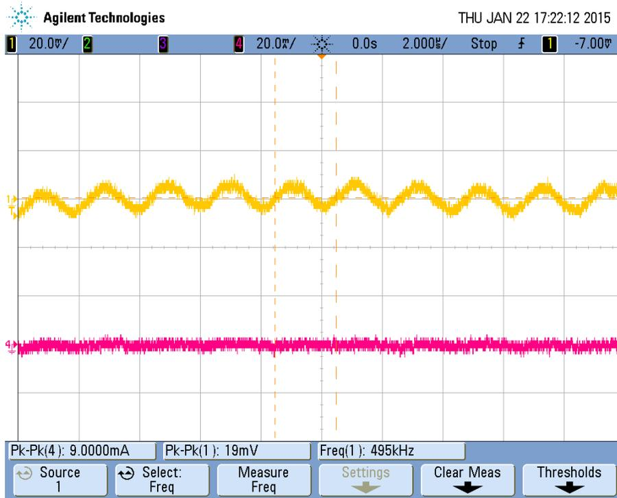
Figure 11 Output ripple at 24Vin, 700mA, 4x LEDs
