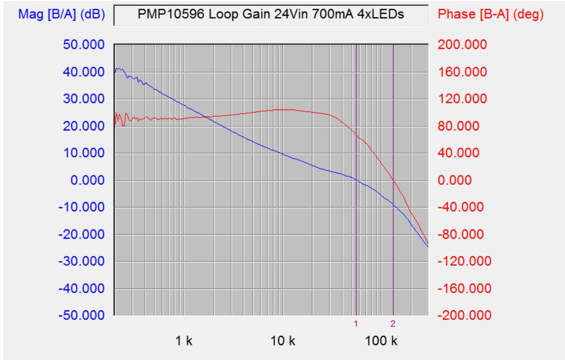
Figure 16 Closed loop response at 24Vin, 700mA, 4x LEDs
