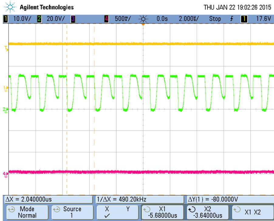
**Figure 14 Open circuit operation at 30Vin**
