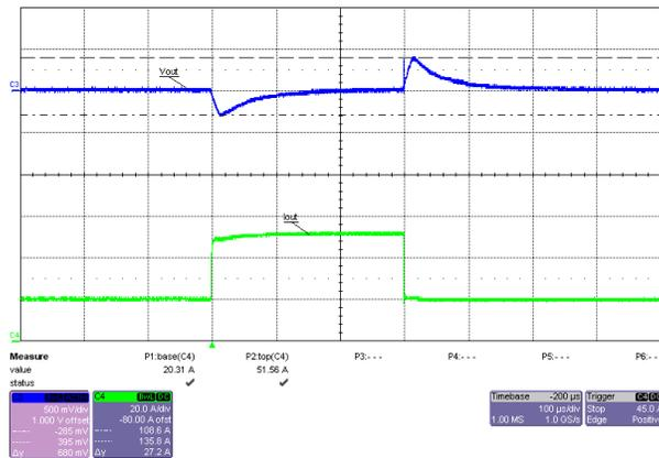
Figure 3-21. Load Transient Response, 60V Input, 20A-to-50A Load Step, FPWM Mode
