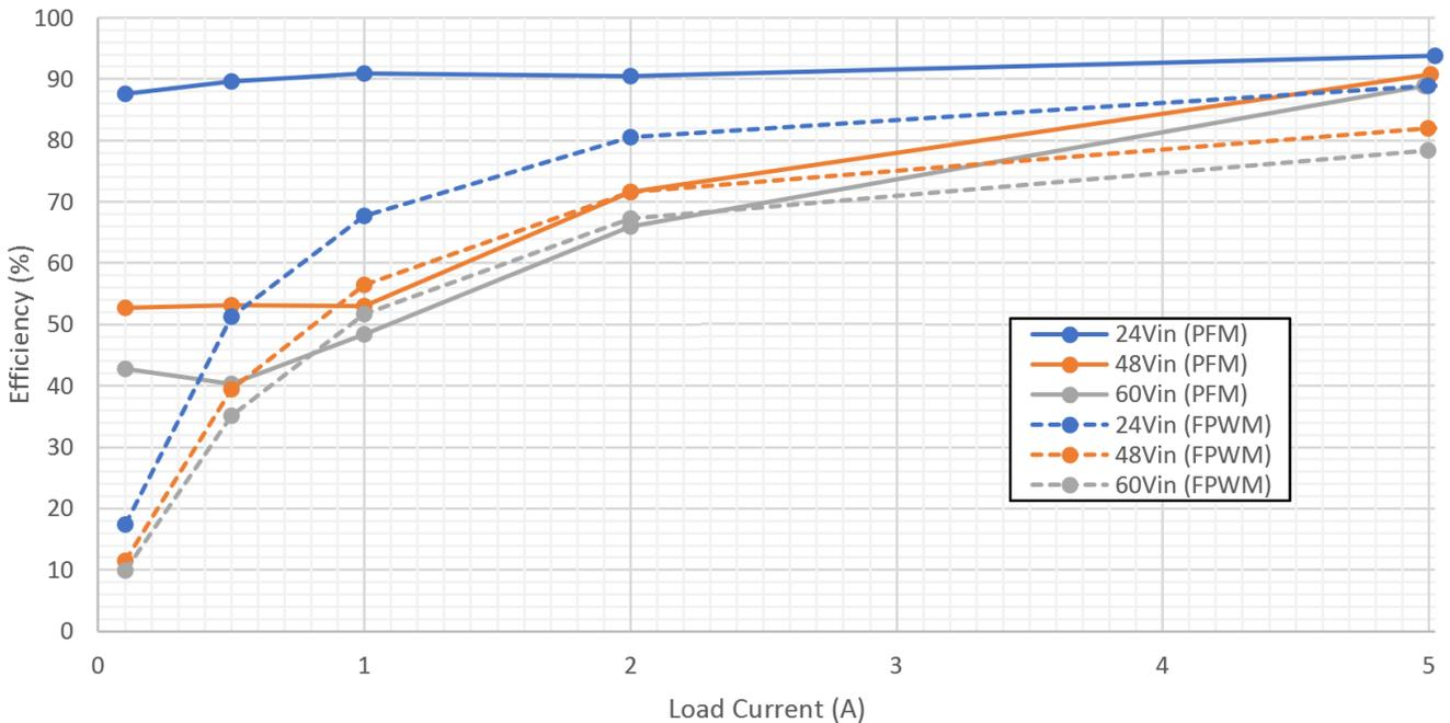
Figure 2-2. Efficiency (0A to 5A)
