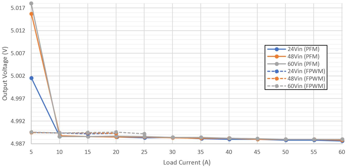
Figure 2-11. Load Regulation (5A to 60A Load)
