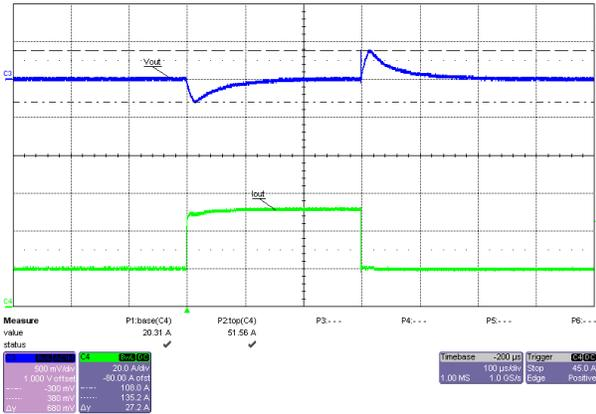
Figure 3-19. Load Transient Response, 24V Input, 20A-to-50A Load Step, FPWM Mode
