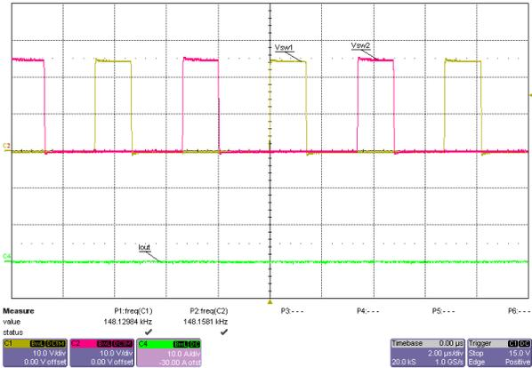
**Figure 3-2. Switch Node Voltages, 24V Input, No Load, FPWM Mode**
