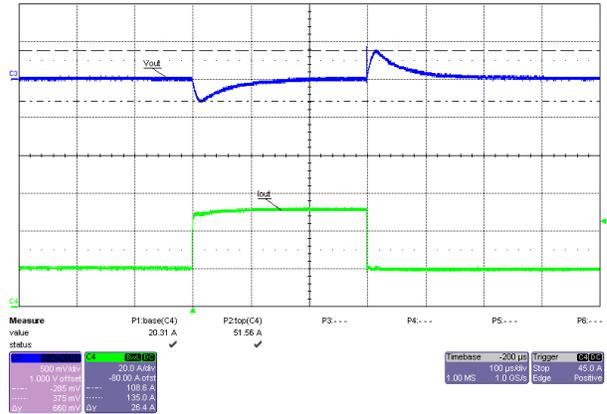
Figure 3-20. Load Transient Response, 48V Input, 20A-to-50A Load Step, FPWM Mode
