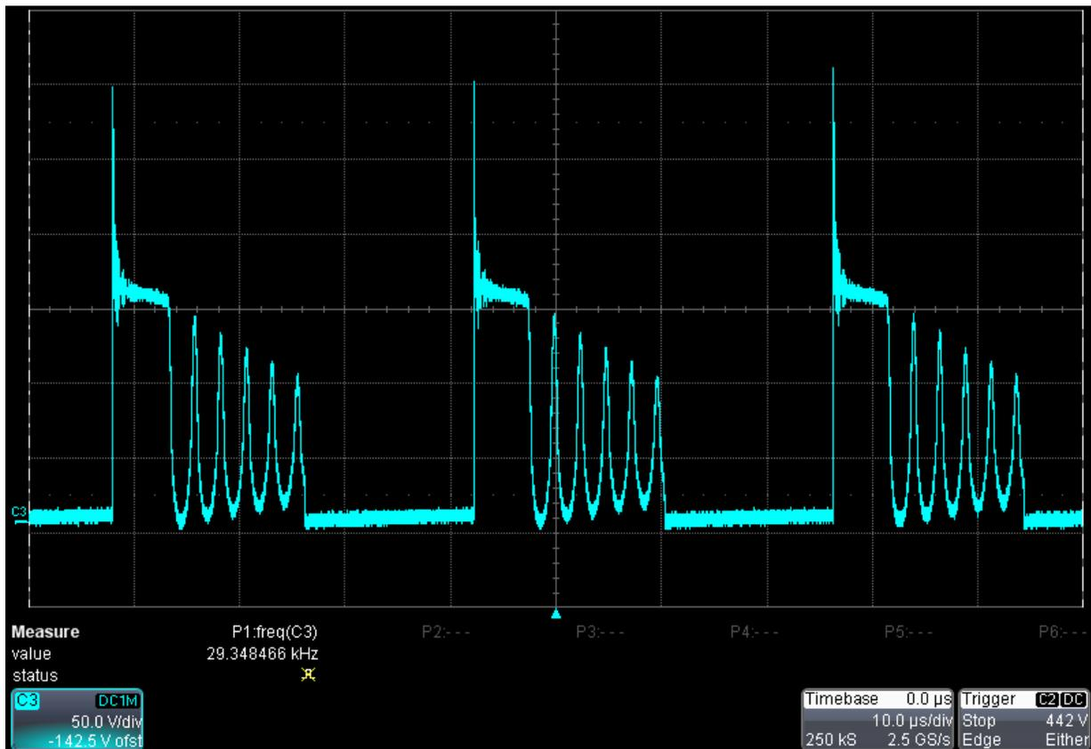
**Figure 9.** Primary Switch Node at 40 Vdc Input, 0.33 A out
