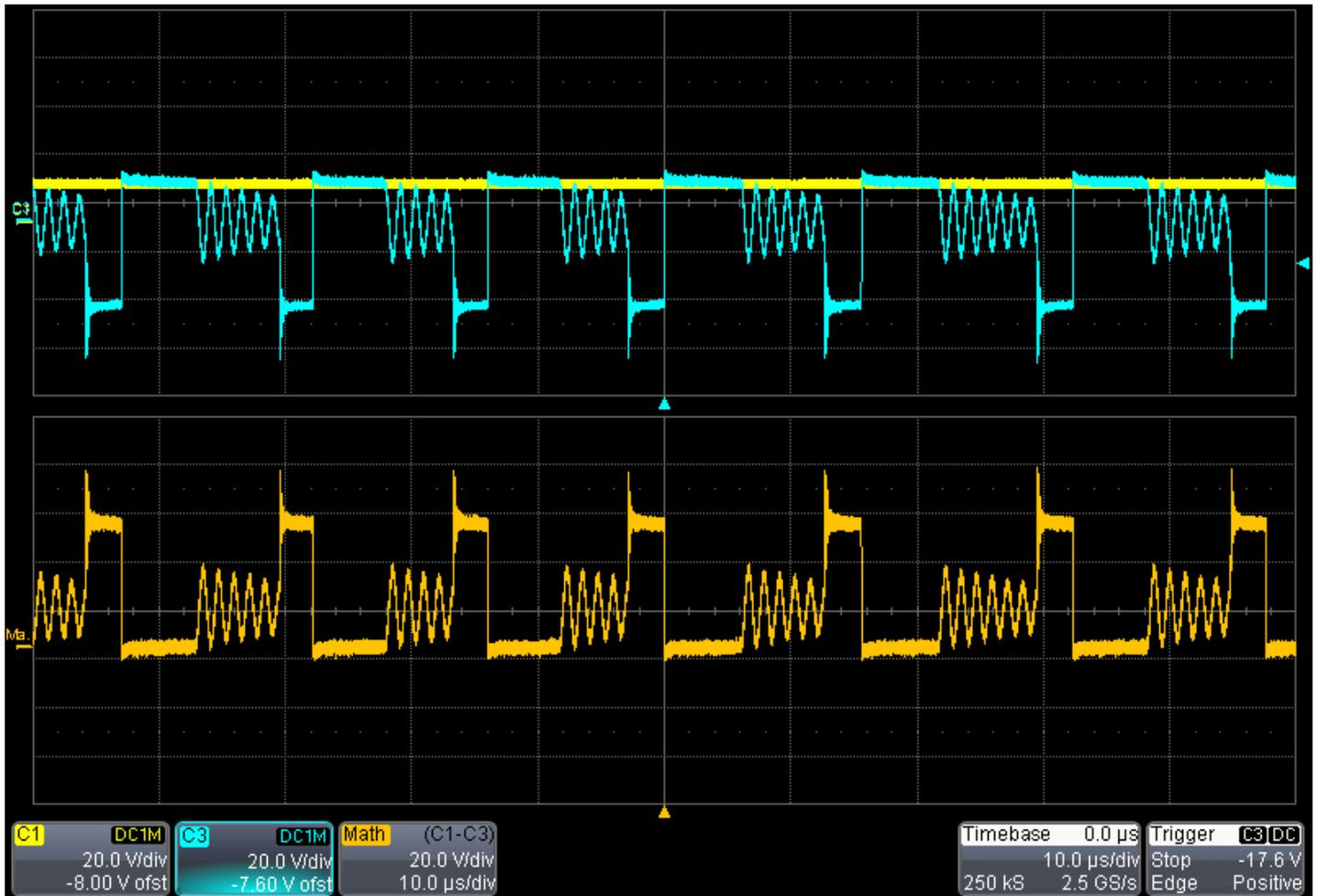
Figure 12. Secondary Switch Node at 250 Vdc Input, 1 A out
