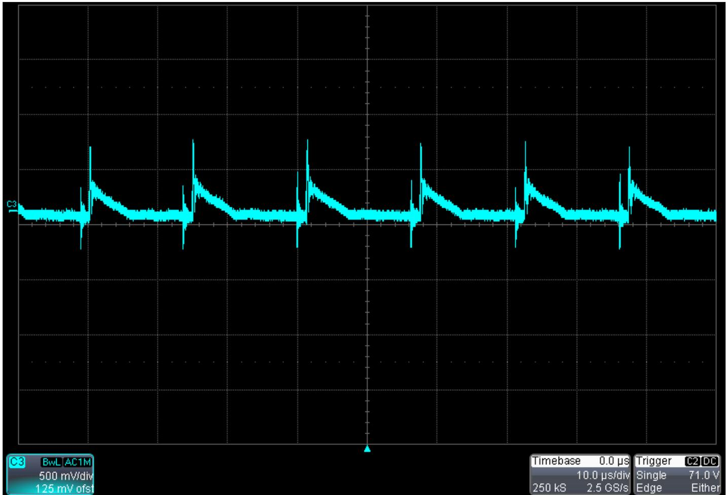
Figure 15. Output Ripple at 550 Vdc Input, 1 A out
