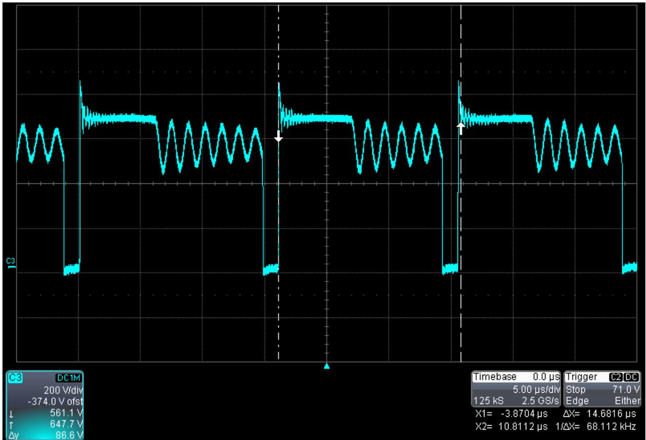
Figure 11. Primary Switch Node at 550 Vdc Input, 1 A out
