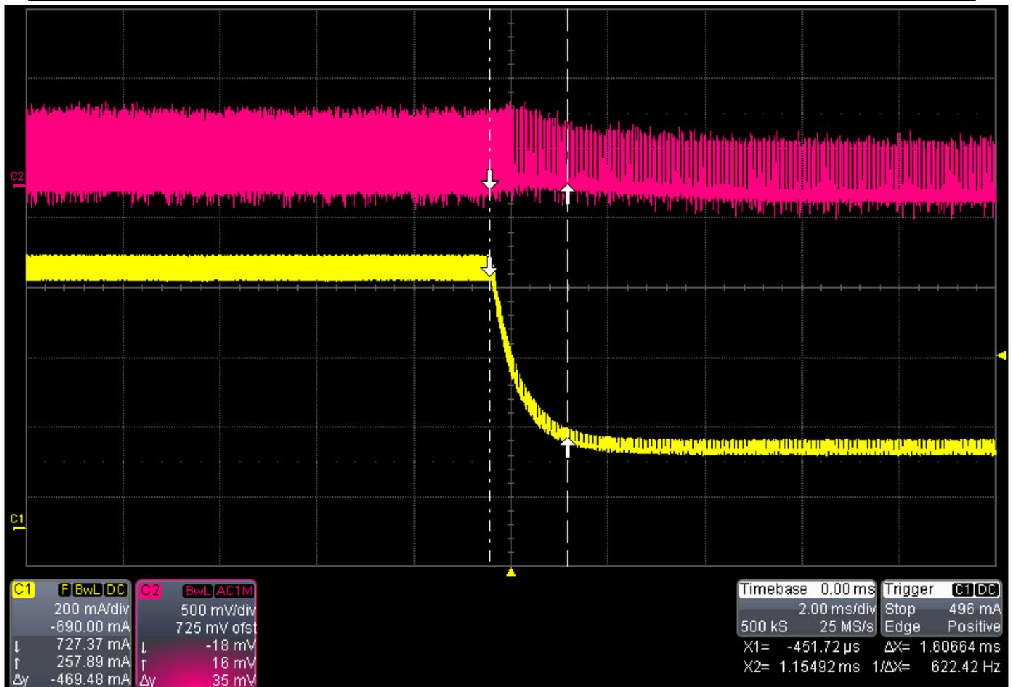
Figure 17. Load transient falling edge, 250V<sub>in</sub>
