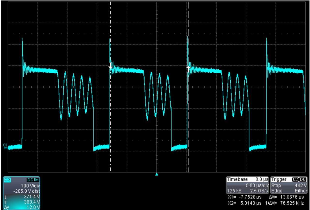
Figure 10. Primary Switch Node at 250 Vdc Input, 1 A out
