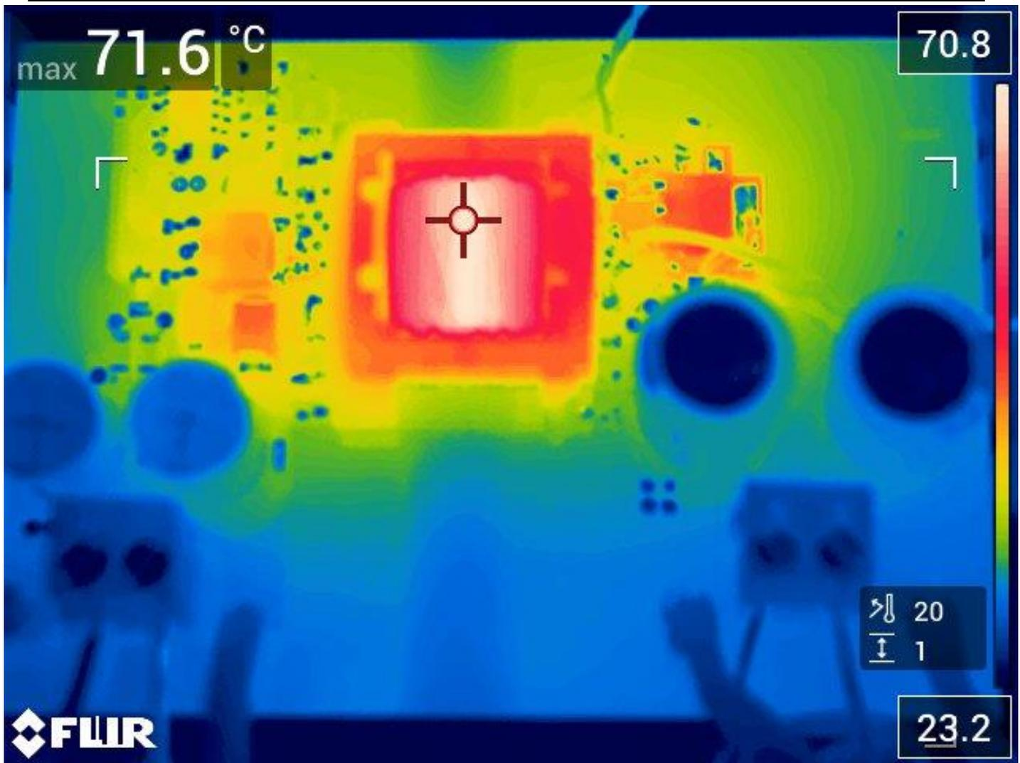
Figure 8. Board top thermal image, 550Vin, 1 A out
