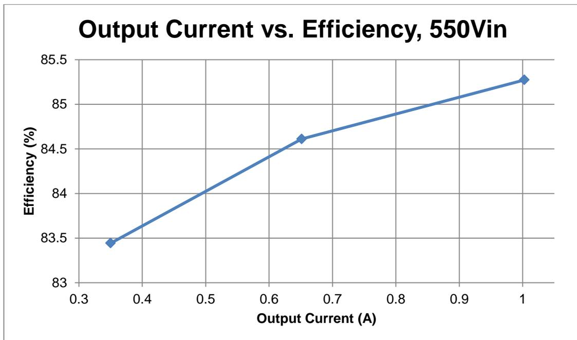
**Figure 4.** Efficiency for 550 Vdc input
