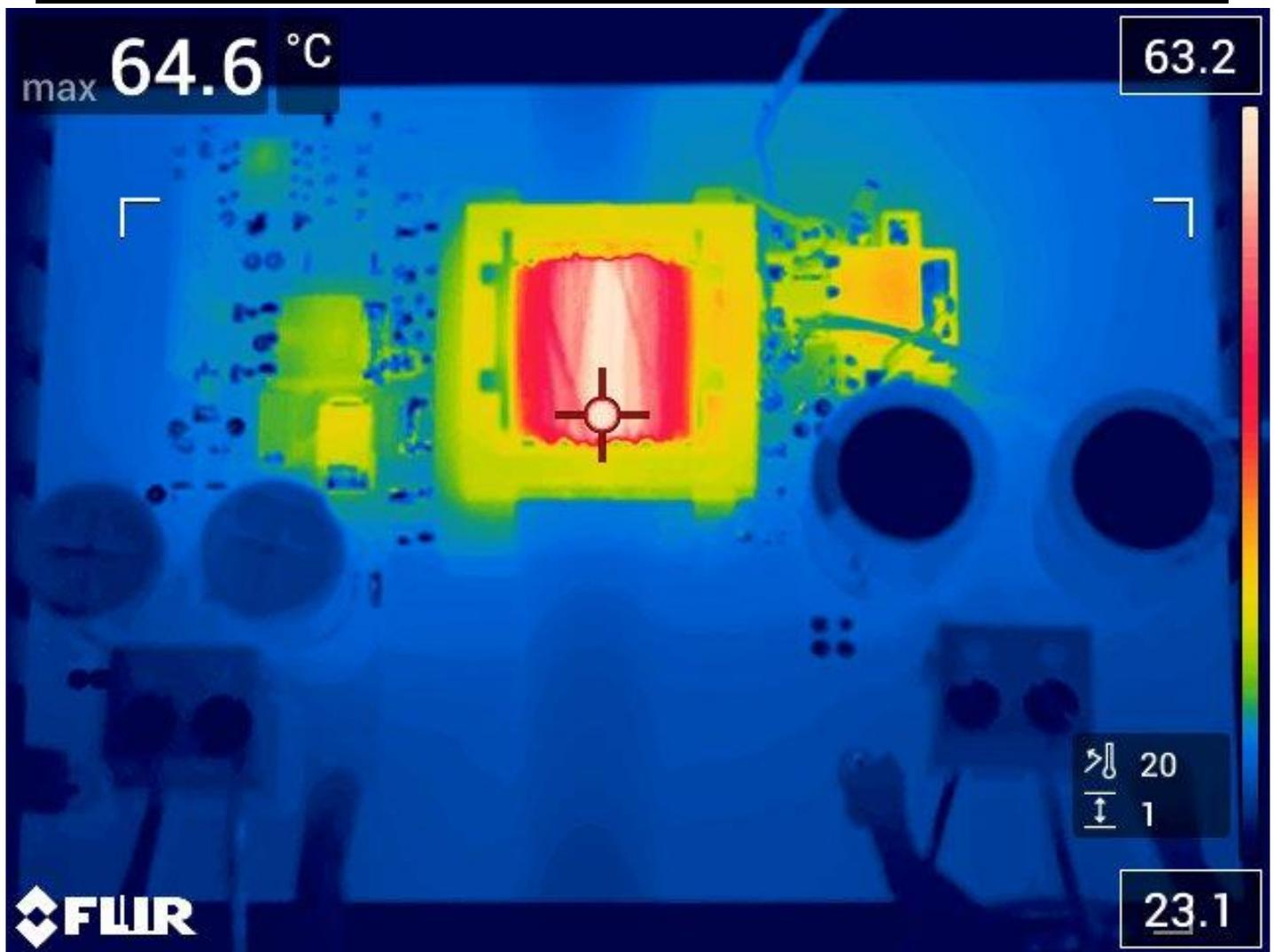
Figure 7. Board top thermal image, 250Vin, 1 A out
