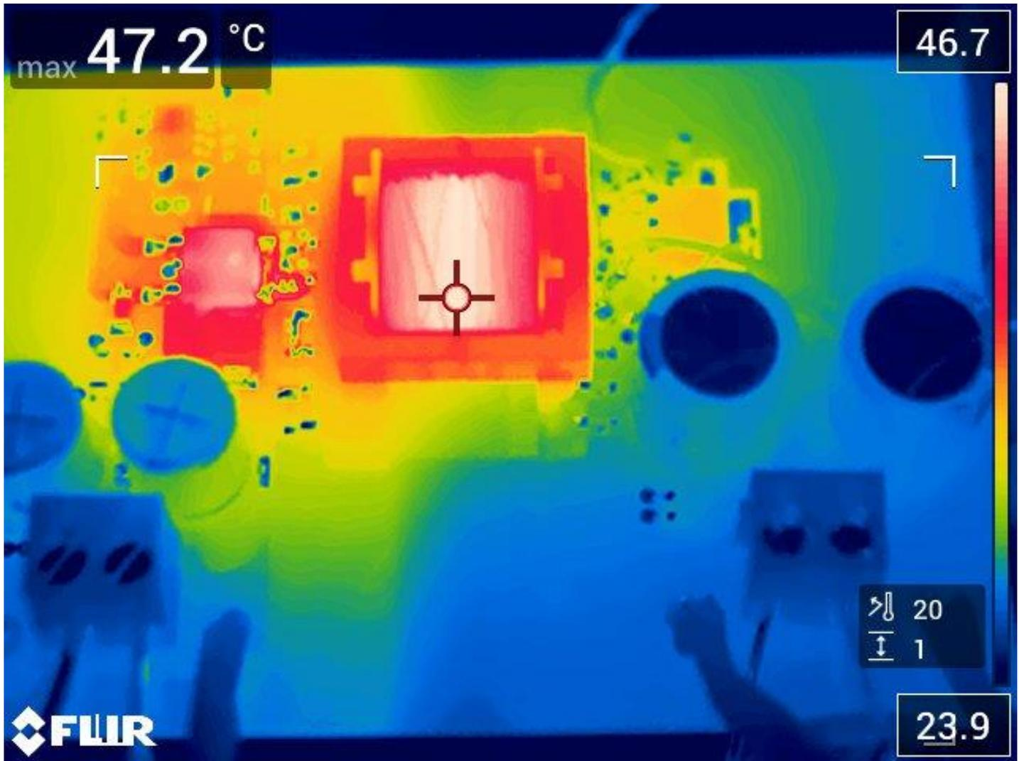
Figure 6. Board top thermal image, 40V<sub>in</sub>, 0.33 A out
