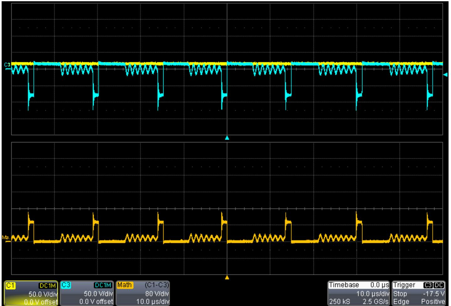
Figure 13. Secondary Switch Node at 550 Vdc Input, 1 A out
