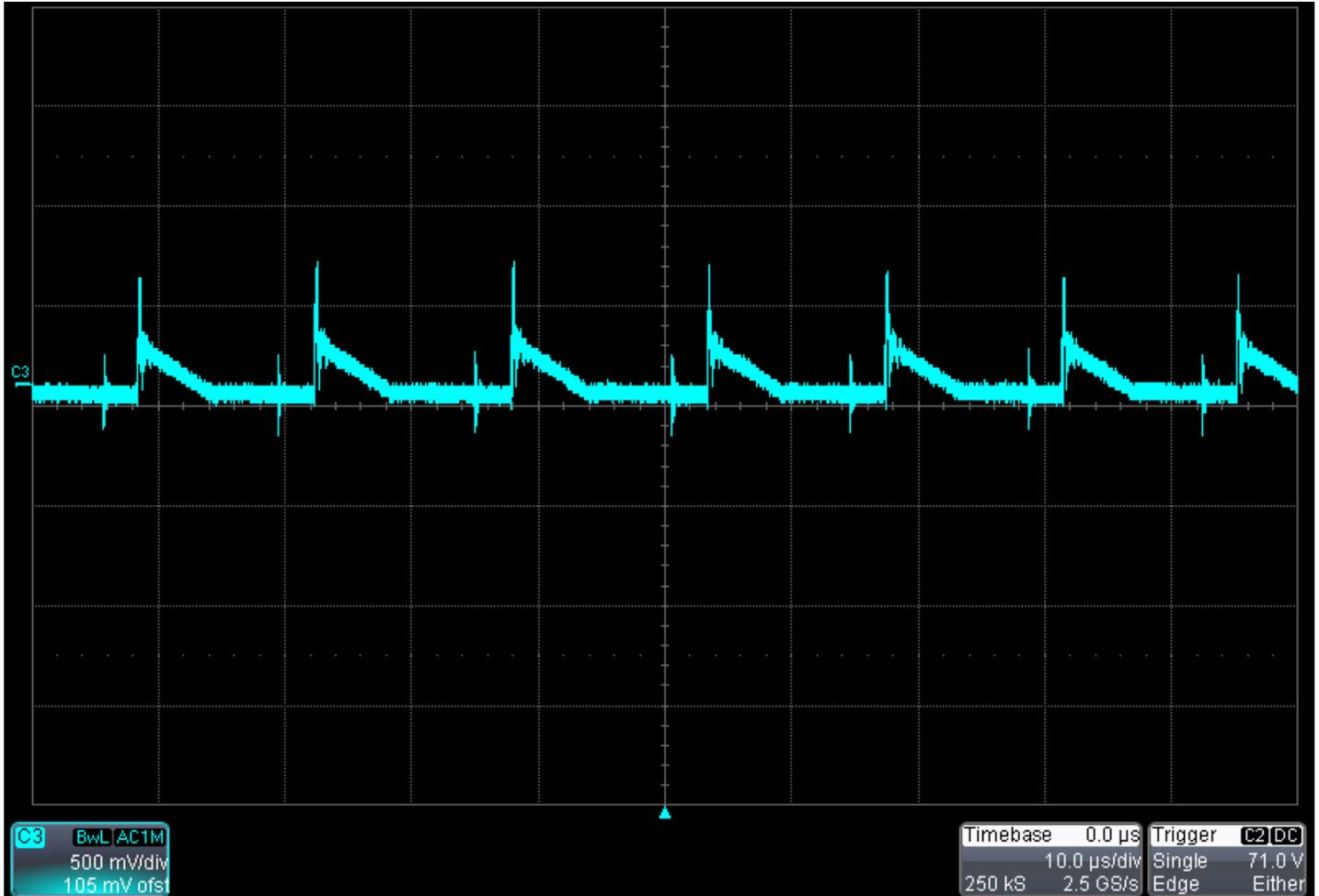
**Figure 14.** Output Ripple at 250 Vdc Input, 1 A out
