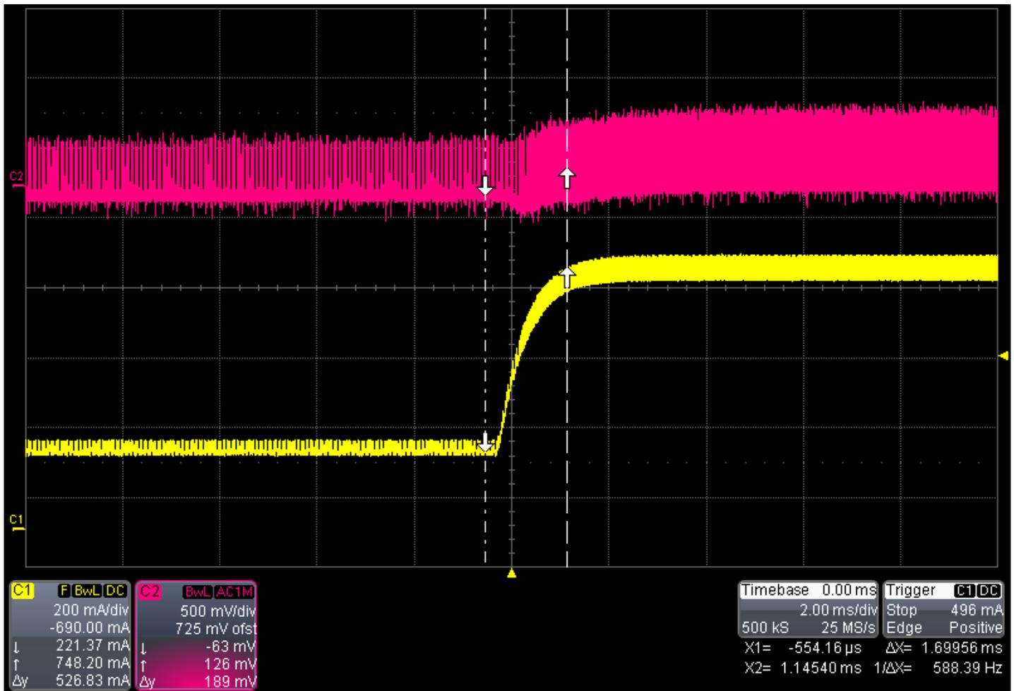
**Figure 16.** Load transient rising edge, 250Vin
