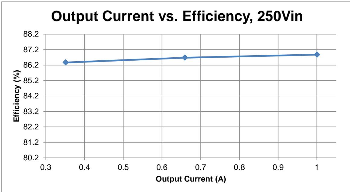
**Figure 3.** Efficiency for 250 Vdc input
