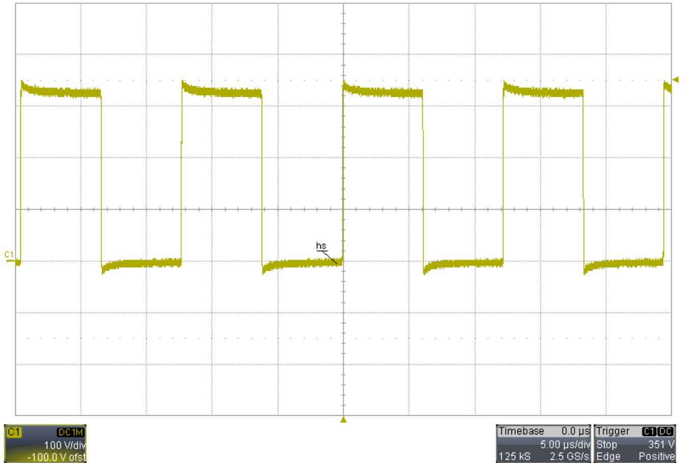
**Figure 8.** Primary Switching Node Waveform
