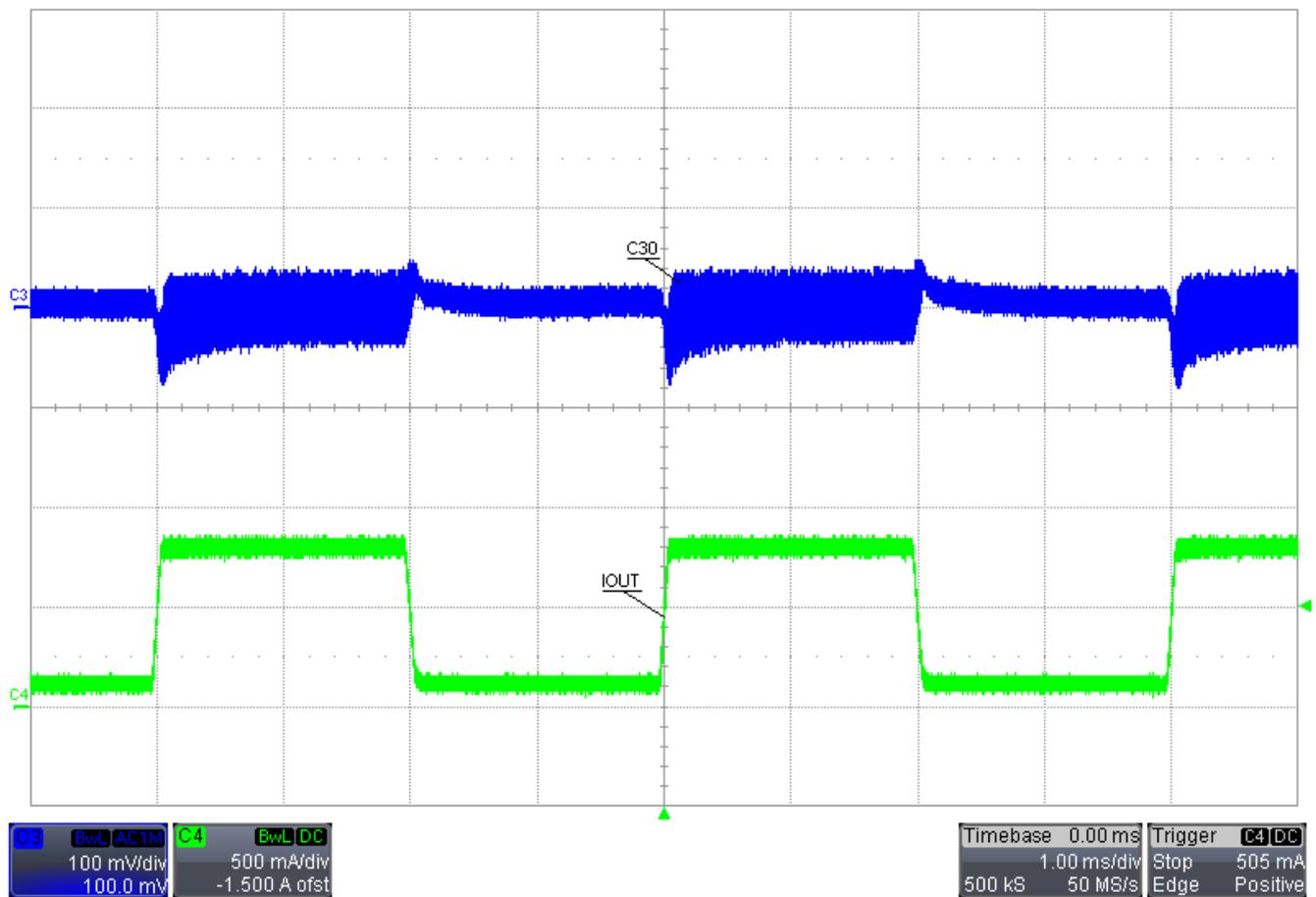
Figure 17. Load Transient on Output 2 (C30). Output current from the 13.8V rail is shown.
