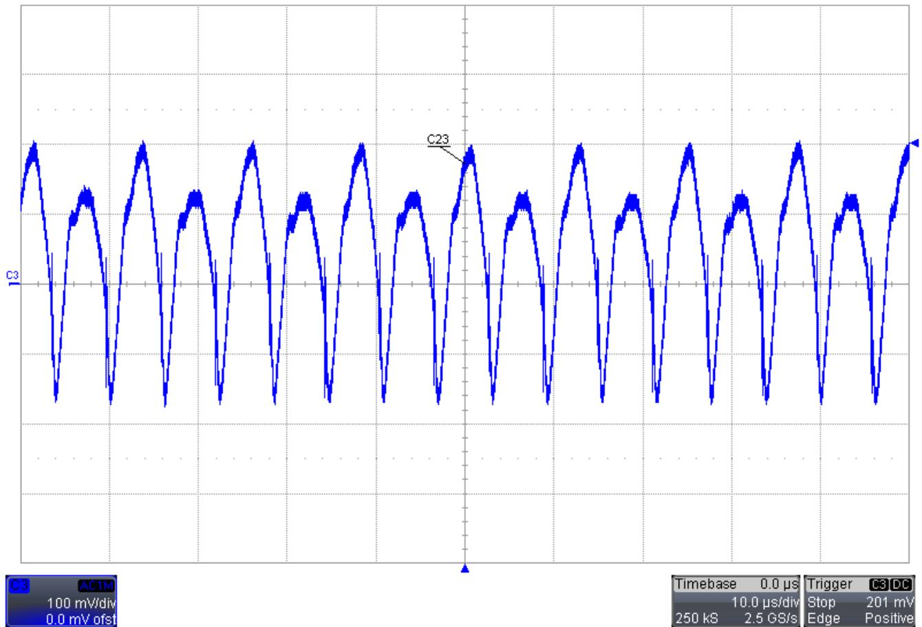
Figure 13. Output 1 Voltage Ripple (C23)
