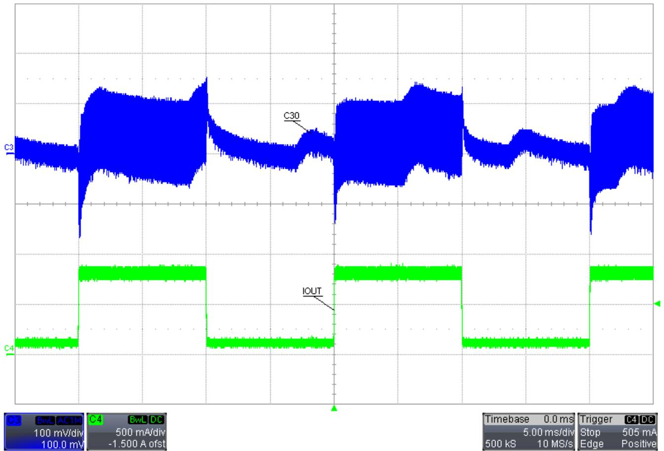
Figure 18. Load Transient on Output 2 (C30). Output current from the 13.8V rail is shown.
