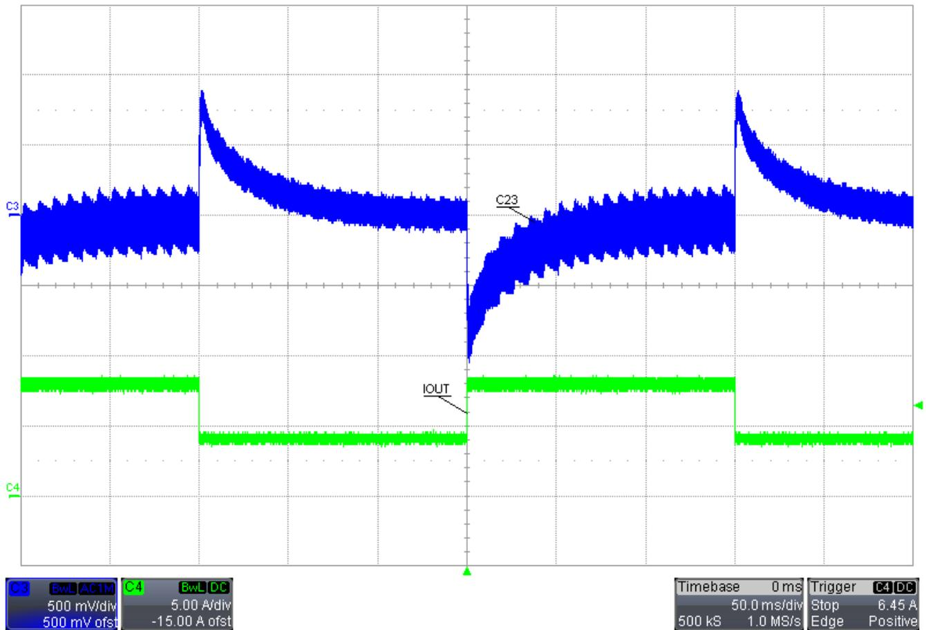
Figure 16. Load Transient on Output 1 (C23). Output current from the 30V rail is shown.
