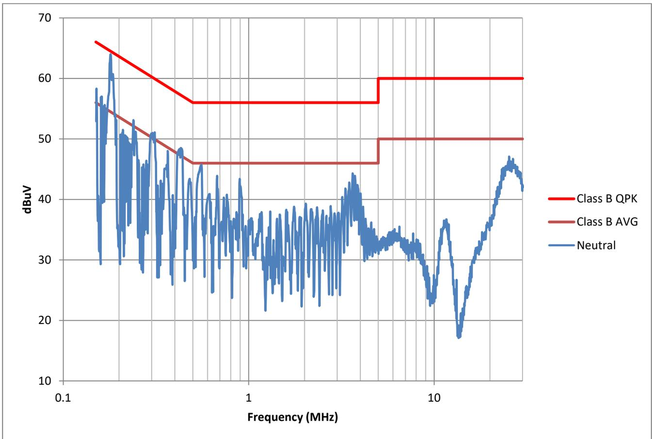
Figure 21. Earthed output, Neutral Measurement
