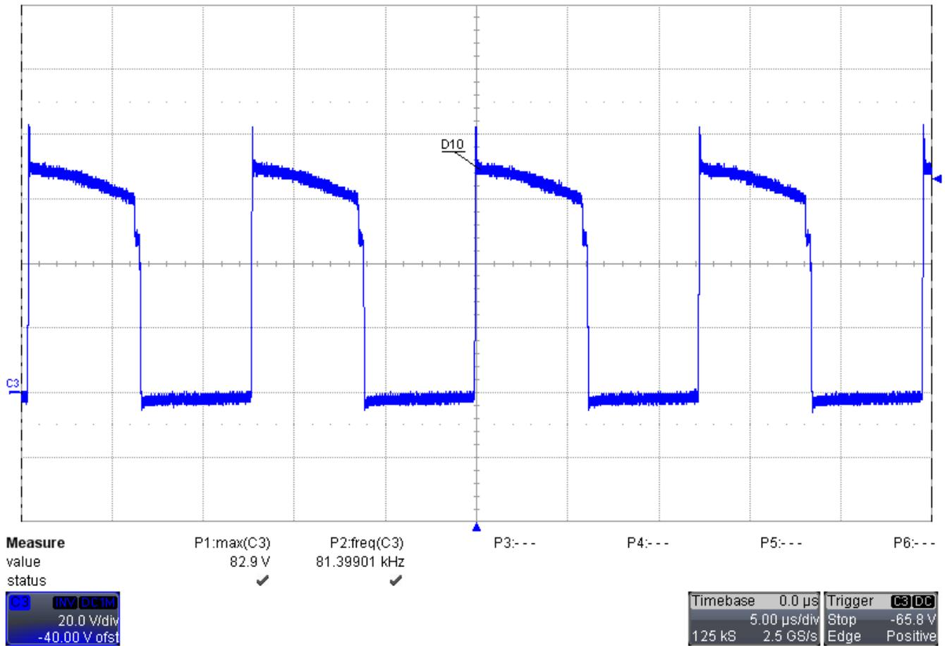
**Figure 12.** Secondary Switching Node Waveform (D10) with persistence mode on oscilloscope
