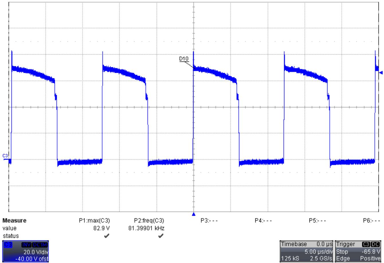
Figure 11. Secondary Switching Node Waveform (D10)
