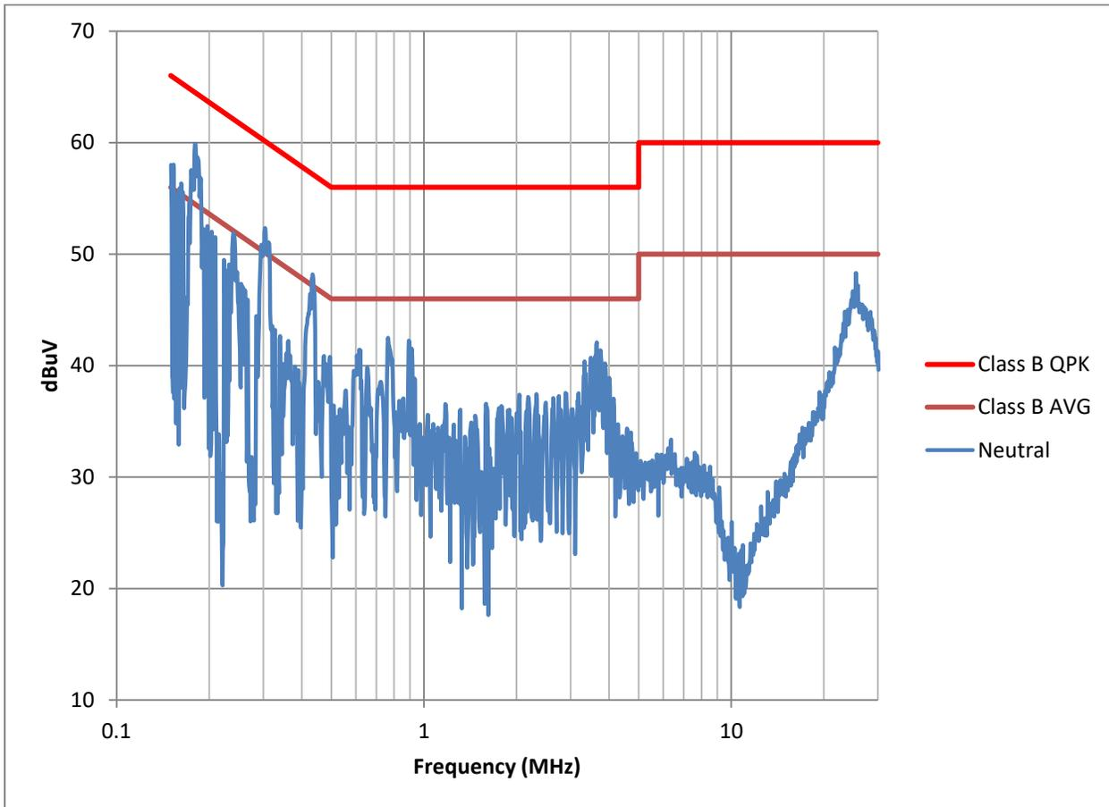
Figure 23. Non-Earthed output, Neutral Measurement
