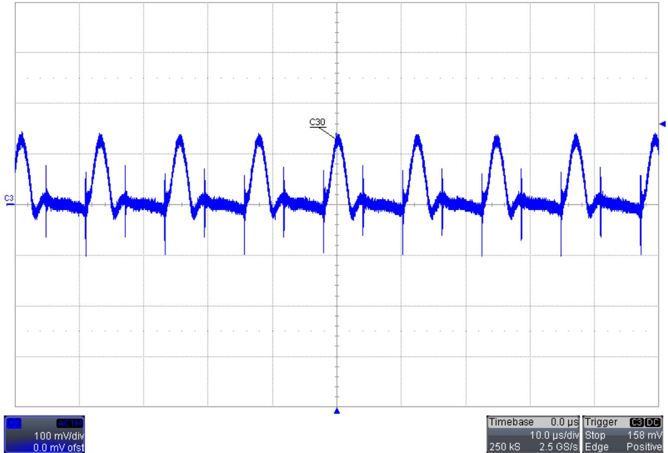
Figure 14. Output 2 Voltage Ripple (C30)
