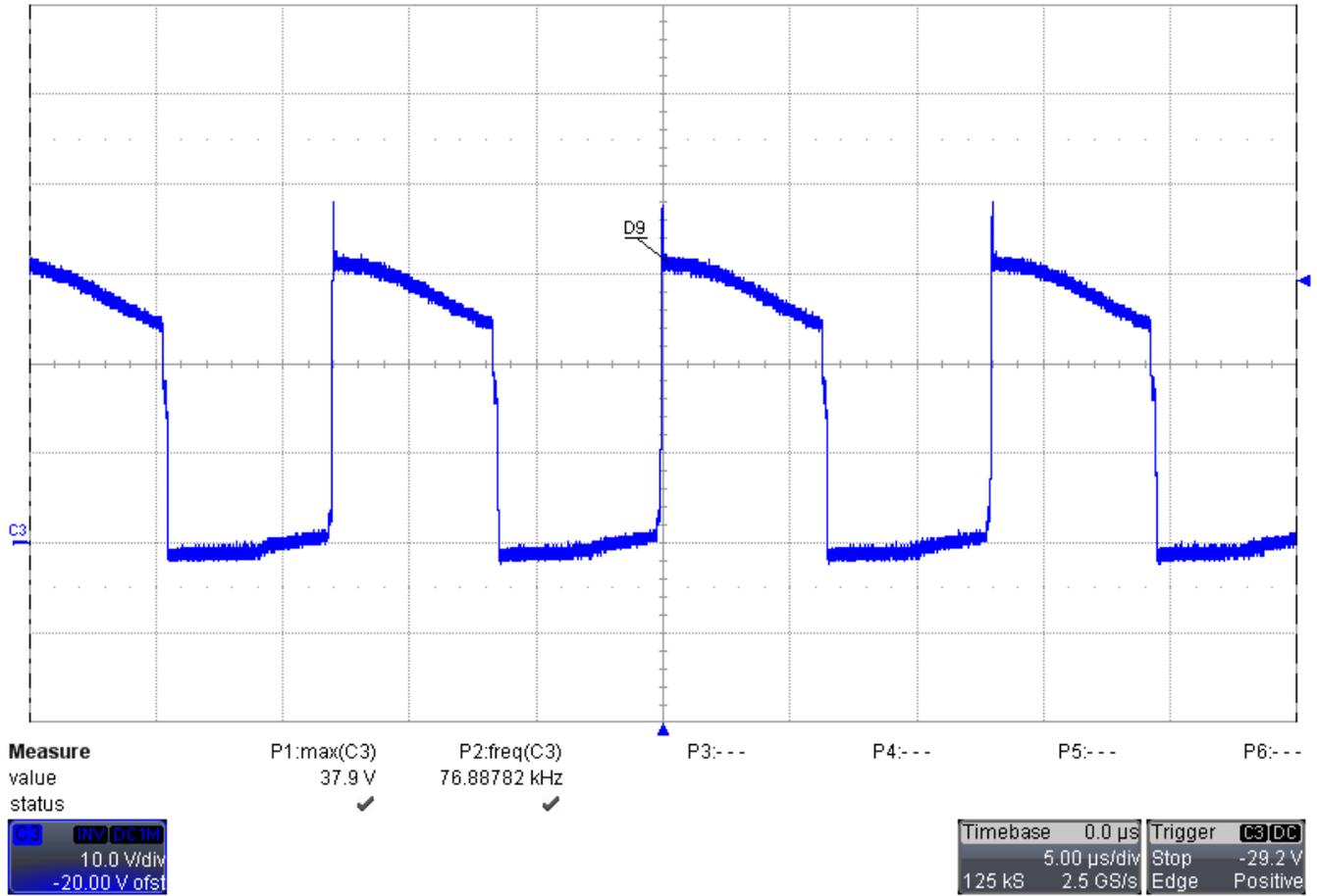
Figure 9. Secondary Switching Node Waveform (D9)
