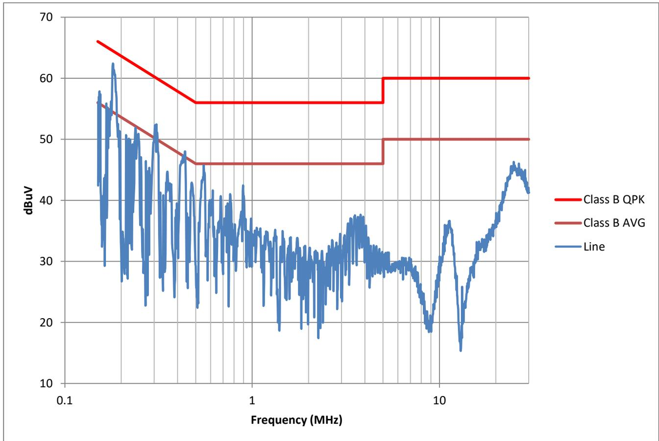
**Figure 20.** Earthed output, Line Measurement
