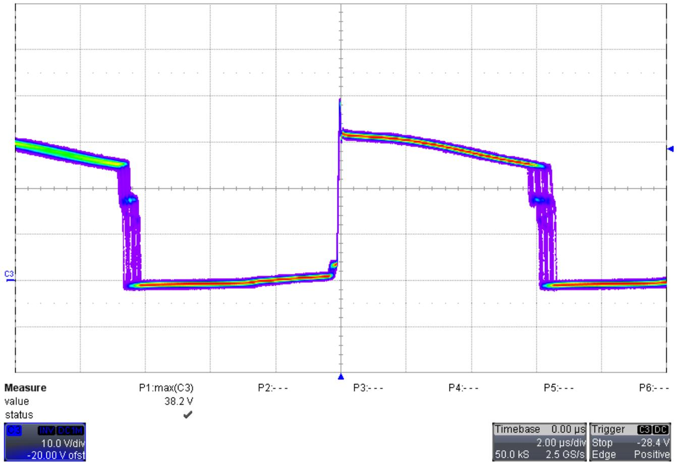
**Figure 10.** Secondary Switching Node Waveform (D9) with persistence mode on oscilloscope
