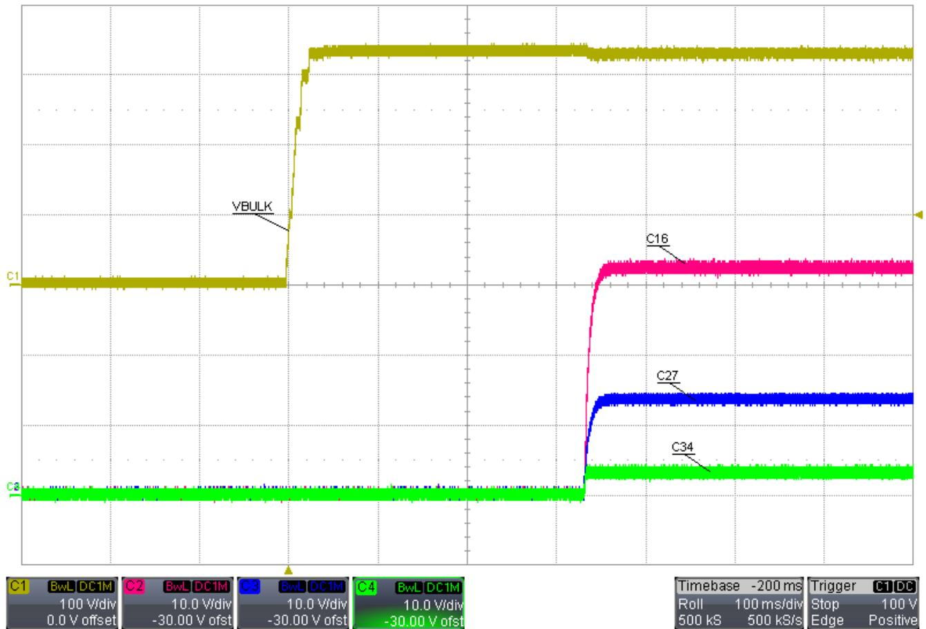
Figure 19. Start up voltages of the input and outputs 1, 2, and 3.
