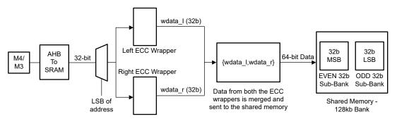
Figure 5-1. Shared Memory Logic Diagram When Shared with M4/M3
