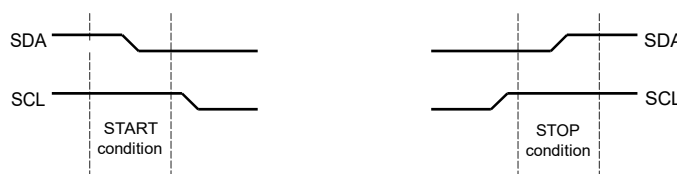
Figure 7-3. START and STOP Conditions
