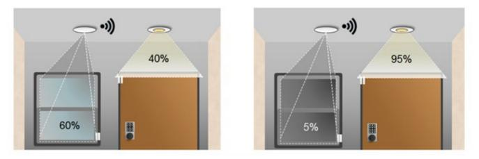
Figure 1. External vs. Artificial Light Intensity Balancing Examples
