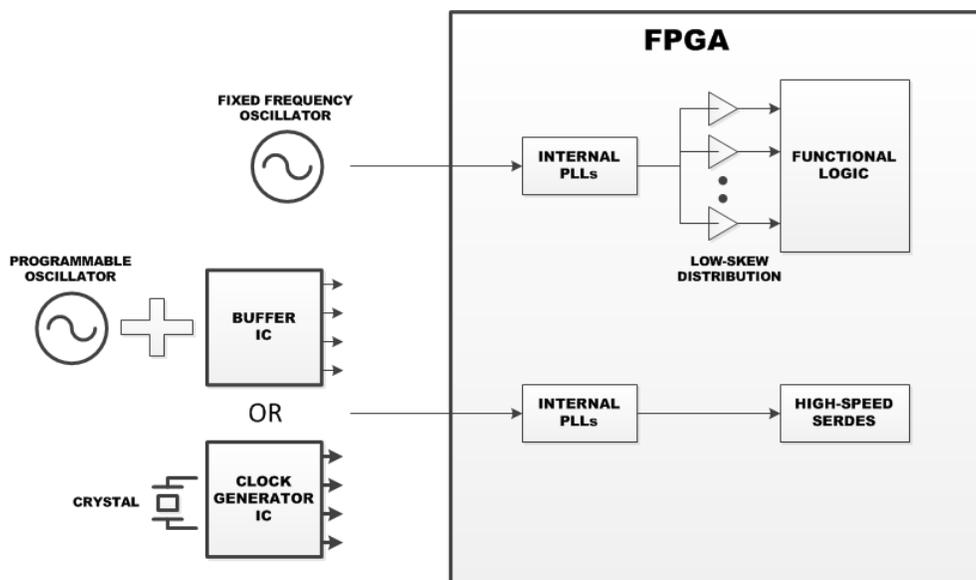
Figure 1. Reference Clocks for FPGAs
