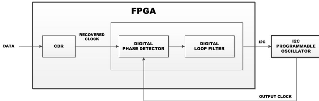
**Figure 2. Digital Controlled Oscillator**
