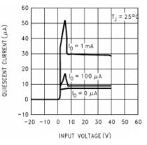
Figure 2. I<sub>Q</sub> For LM2936
