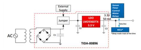
Figure 1. TIDA-00896 High-level Block Diagram
