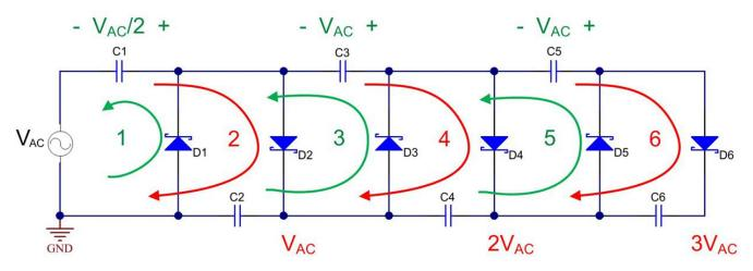
Figure 1. A Voltage Multiplier Uses an Alternating Current (AC) Voltage with Diodes and Capacitors in a Cascade
