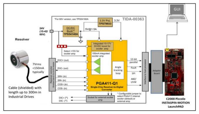
Figure 1. Simplified System Block Diagram of the TIDA-00363 Reference Design with F28069M MCU LaunchPad<sup>™</sup> Development Kit
