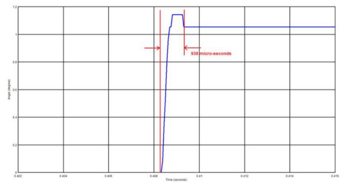
Figure 2. Step Response for 1-Degree Angle Change
