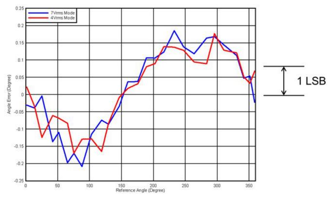
Figure 3. Angle Error with 7Vrms and 4Vrms Excitation Modes
