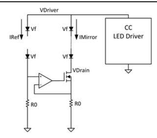
Figure 6. Open Circuit in the Reference String
