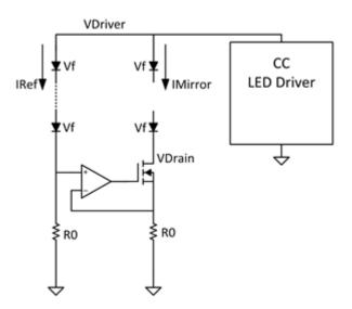
Figure 5. Open Circuit in the Mirror String
