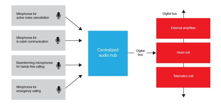
Figure 4. A centralized audio hub module
