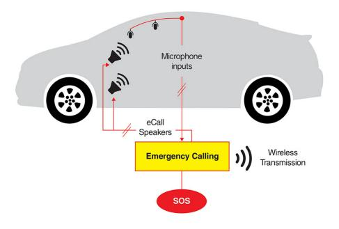
Figure 3. How an eCall System Works
