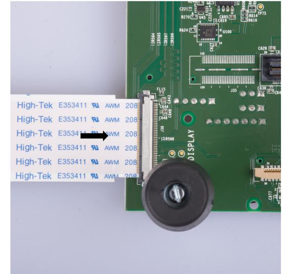
Note that if you need to pull the flex cable off, you can do so by simultaneously pressing on the connector metal strip and pulling the flex cable.
