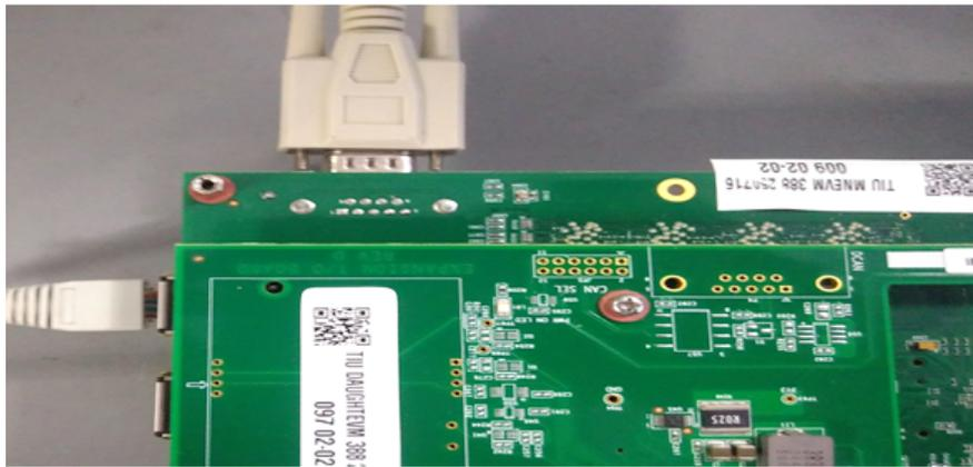
**Figure 4. Serial Cable Connected to EVM**
