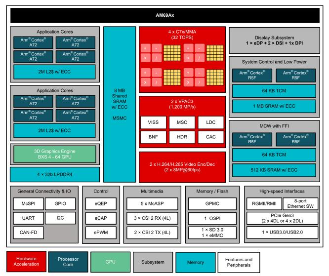
Figure 2-1. AM69A Block Diagram With Subsystems
