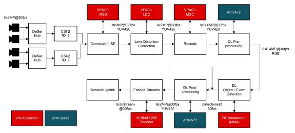
Figure 3-3. Multi-Camera Al Block Diagram With Data Flow on AM69A
