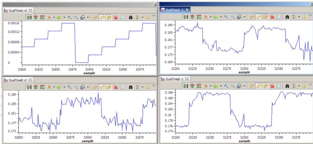
**Figure 5 Graph Windows for Build Level 1 (a) mod6 counter, (b) BemfA, (c) BemfB and (d) BemfC**
