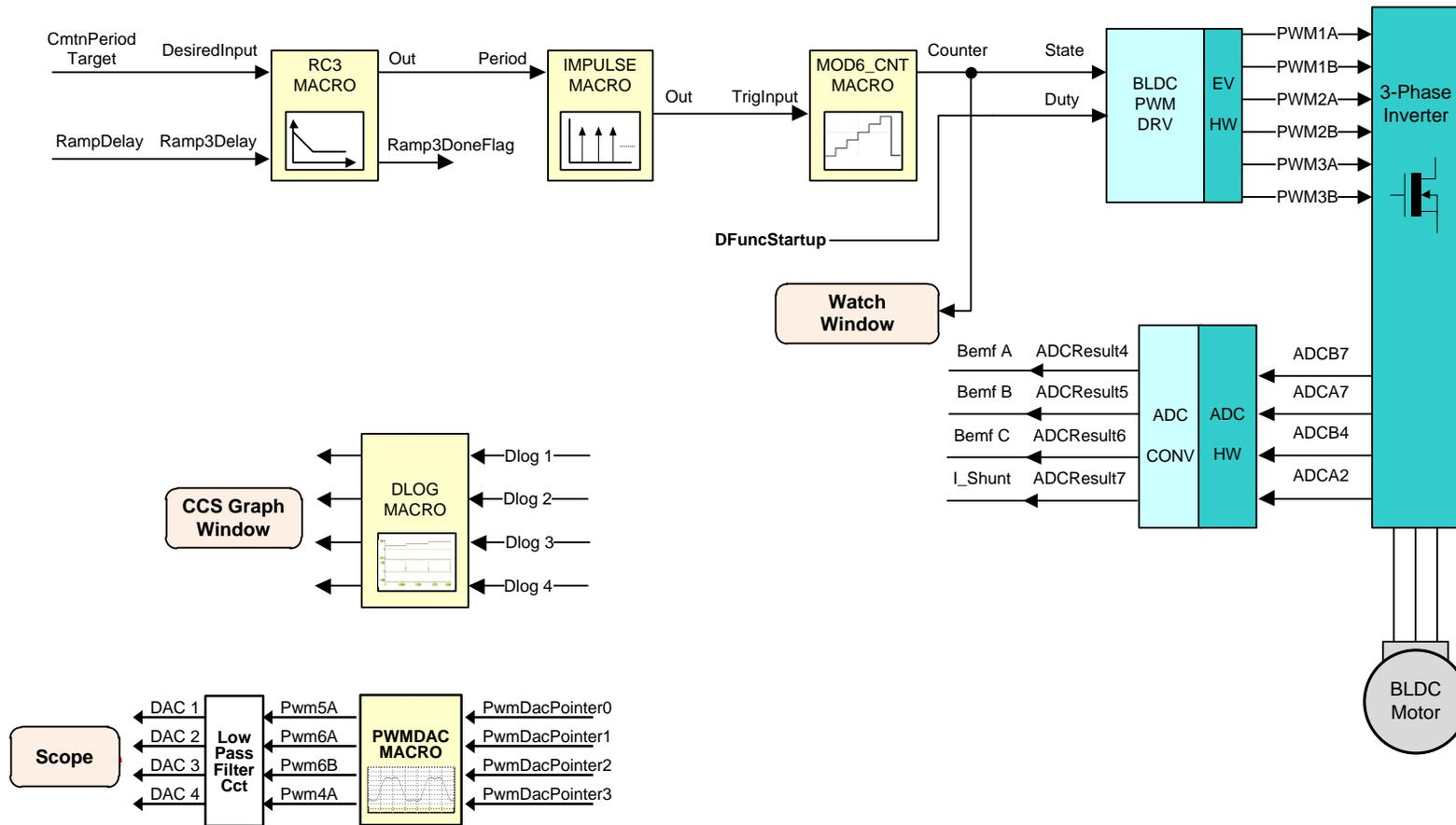
Level 2 verifies the open loop motor operation and current measurement.
