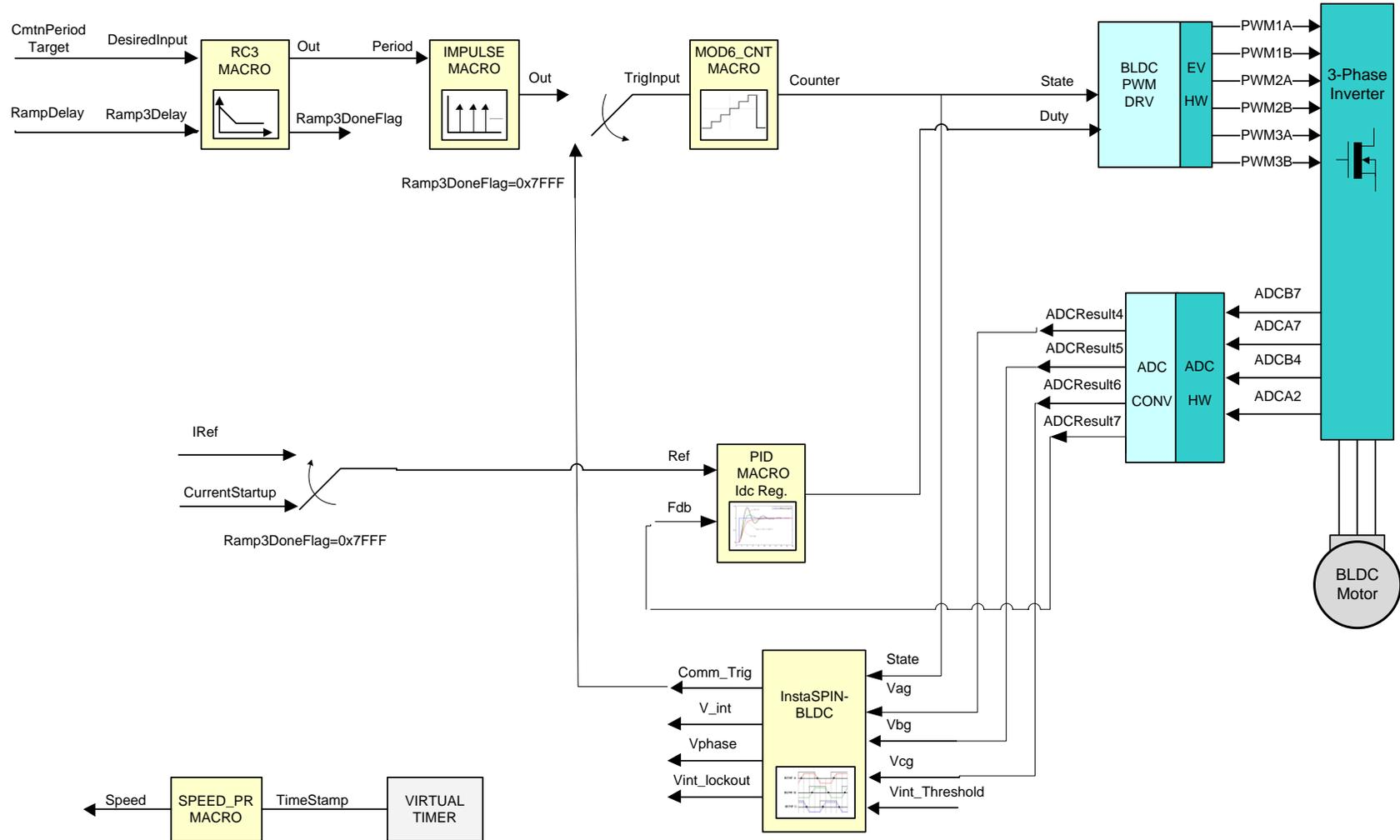
Level 6 verifies the closed current loop and current PI controller.
