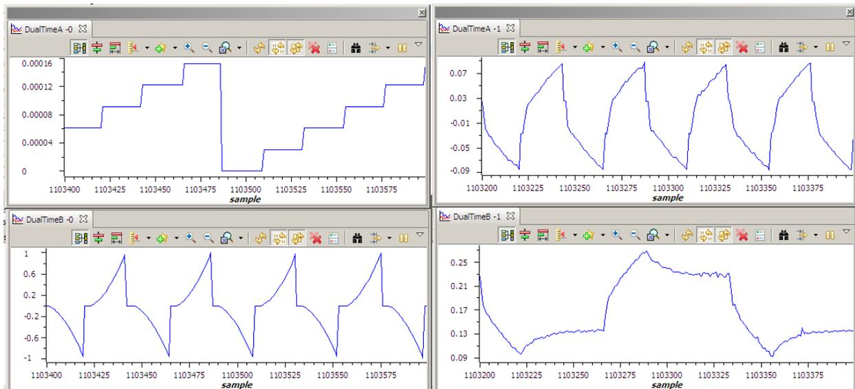
Figure 12 Graph Windows for Build Level 8 (a) mod6 counter, (b) V\_int, (c) Vphase and (d)Vag
