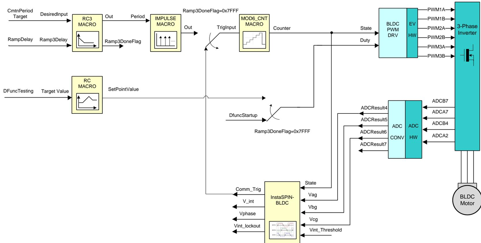
Level 5 verifies the closed loop motor operation based on InstaSPIN-BLDC and the resulting commutation trigger points.
