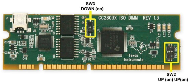
**Figure 33 controlCARD DIP Switch Settings**
