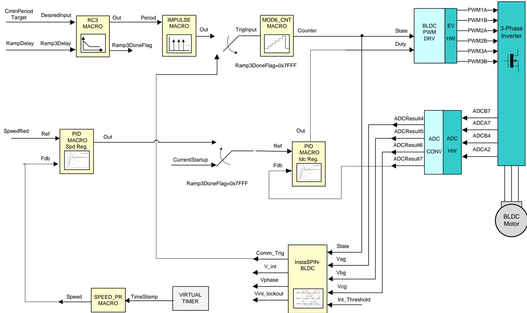
Level 8 verifies the cascaded closed speed and current loops.
