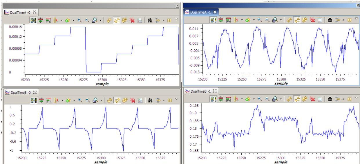
**Figure 8 Graph Windows for Build Level 4 (a) mod6 counter, (b) V\_int, (c) Vphase and (d) Vag**
