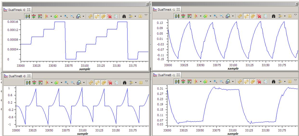
Figure 10 Graph Windows for Build Level 6 (a) mod6 counter, (b) V\_int, (c) Vphase and (d)Vag
