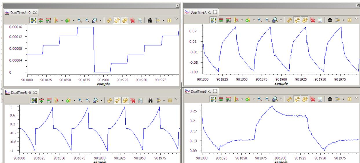
Figure 11 Graph Windows for Build Level 7 (a) mod6 counter, (b) V\_int, (c) Vphase and (d)Vag
