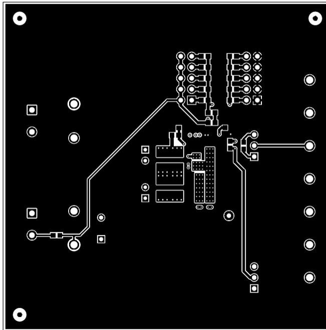
Figure 11. Bottom-Side Copper (Top View)
