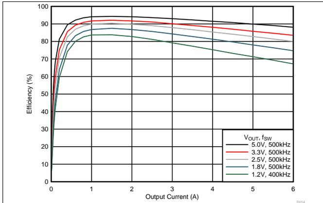
Figure 2. Efficiency ( $V_{in} = 12V$ , FPWM Mode)
