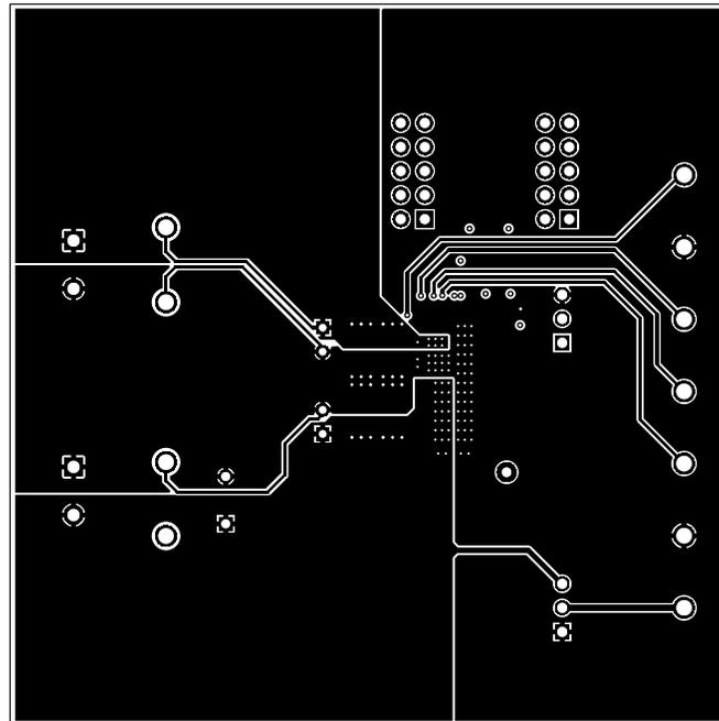
**Figure 10. Layer 3 Copper (Top View)**
