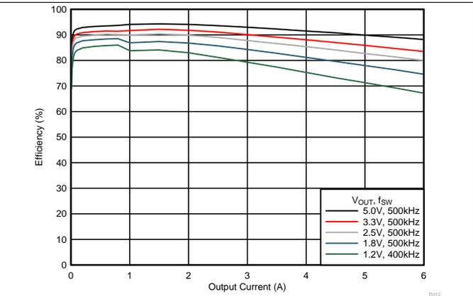
Figure 3. Efficiency ( $V_{in} = 12V$ , Auto Mode)
