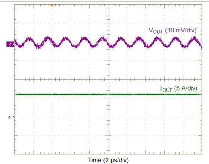
Figure 5. Output Voltage Ripple
