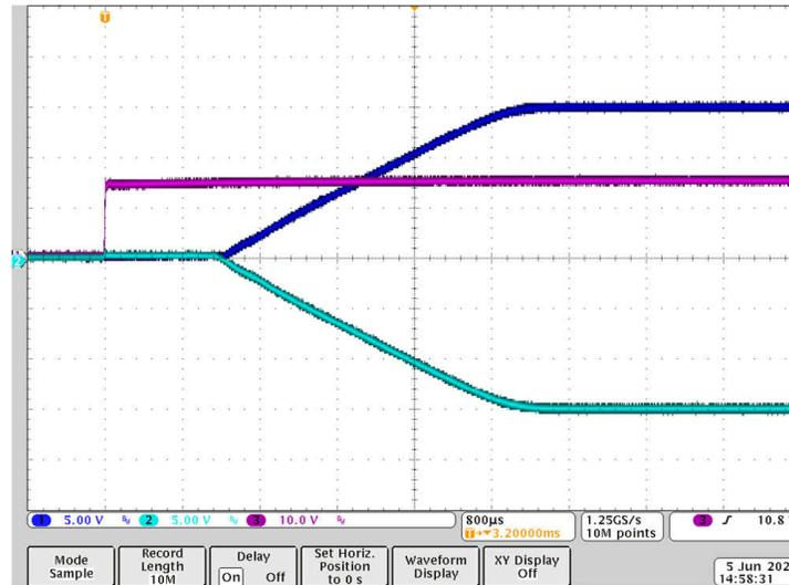
Figure 3-1. Start-up Behavior of Fly-Buck-Boost Topology
