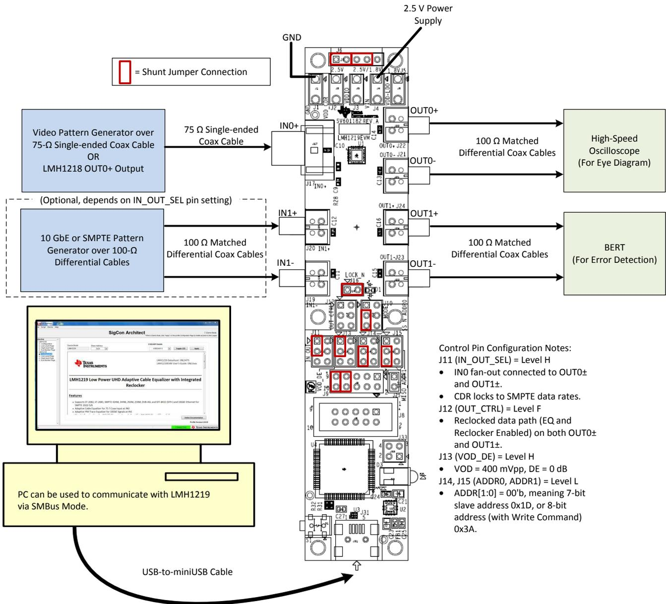
Figure 4. LMH1219EVM Default Setup for Single Supply and SMBus Operation with SigCon Architect
