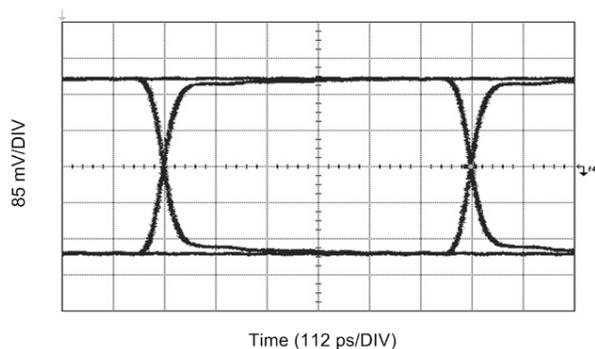
**Figure 9. OUT0 Retimed Output with Belden 1694A Input Cable on IN0+ at 1.485 Gbps**
