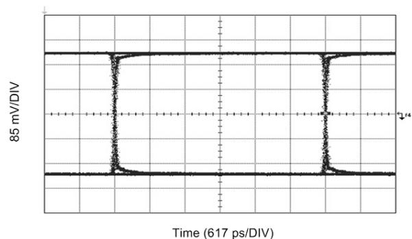
**Figure 10. OUT0 Retimed Output with Belden 1694A Input Cable on IN0+ at 270 Mbps**
