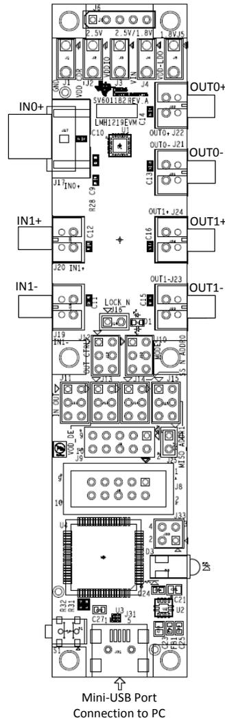
**Figure 2. LMH1219EVM Input and Output Pins**
