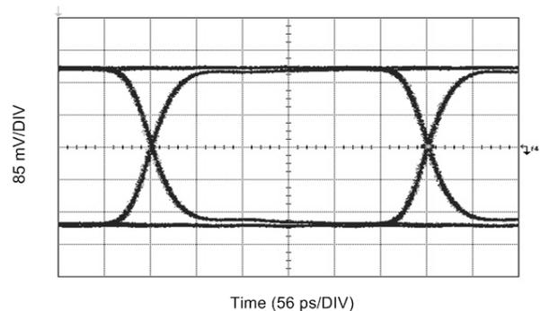
**Figure 8. OUT0 Retimed Output with Belden 1694A Input Cable on IN0+ at 2.97 Gbps**
