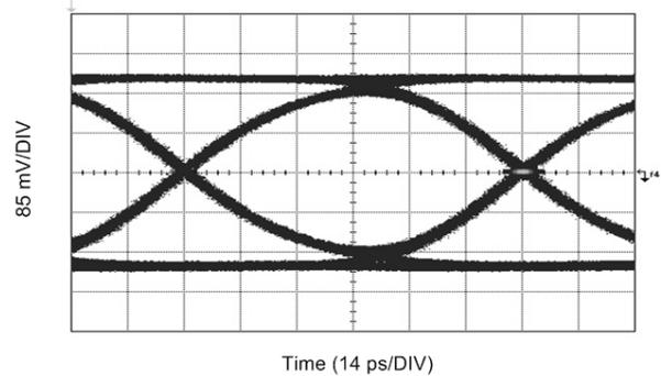
**Figure 6. OUT0 Retimed Output with Belden 1694A Input Cable on IN0+ at 11.88 Gbps**
