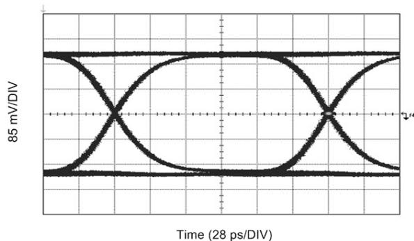
**Figure 7. OUT0 Retimed Output with Belden 1694A Input Cable on IN0+ at 5.94 Gbps**
