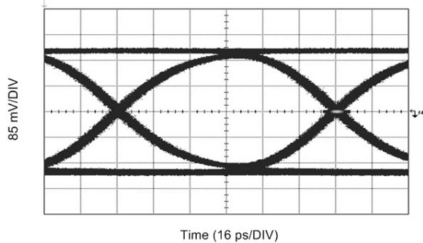
**Figure 5. OUT0 Retimed Output with FR4 Input Trace on IN1± at 10.3125 Gbps**
