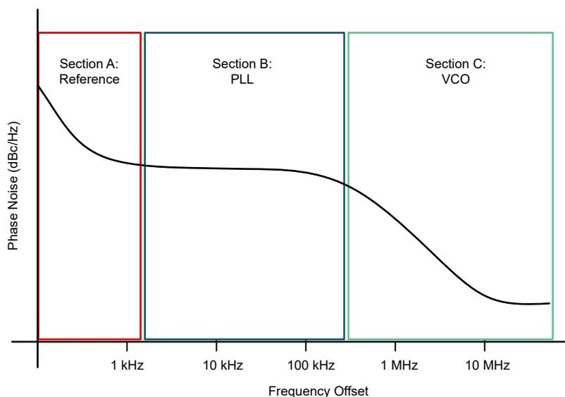
**Figure 1-1. Phase Noise Breakdown by Section**
