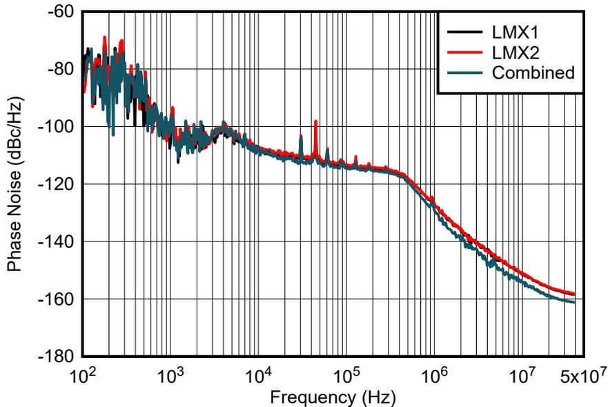
**Figure 2-2. Combined LMX2820 Phase Noise Performance**
