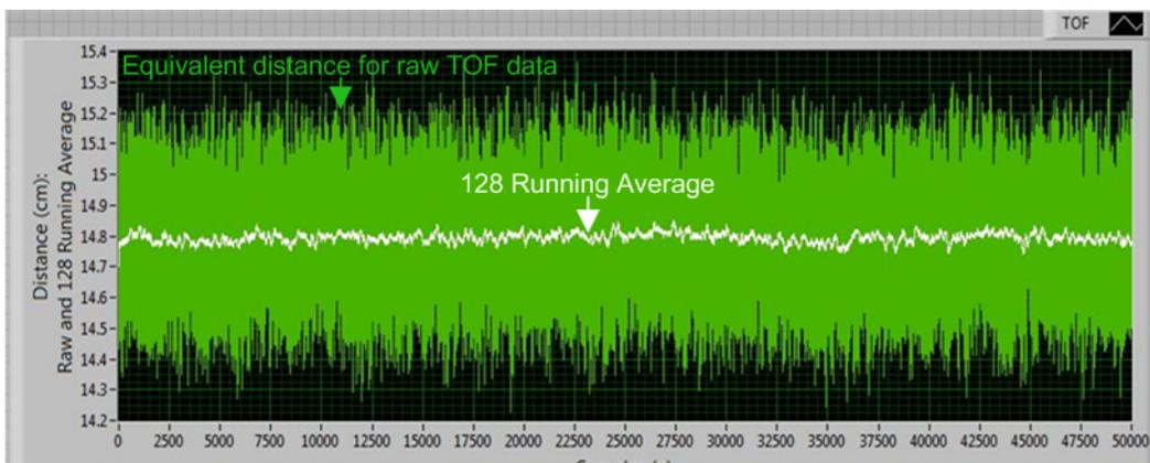
**Figure 17. TDC7201 Combined Measurement Data for TOF=1.0ns: Equivalent Distance Raw and 128x Running Average**
