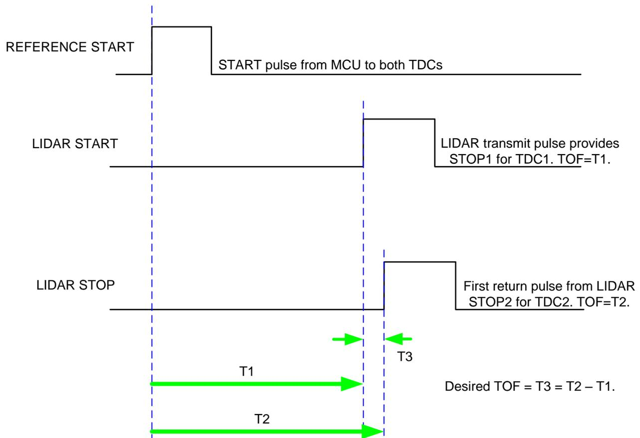
**Figure 6. TDC7201 Short Time Measurements Timing Diagram**
