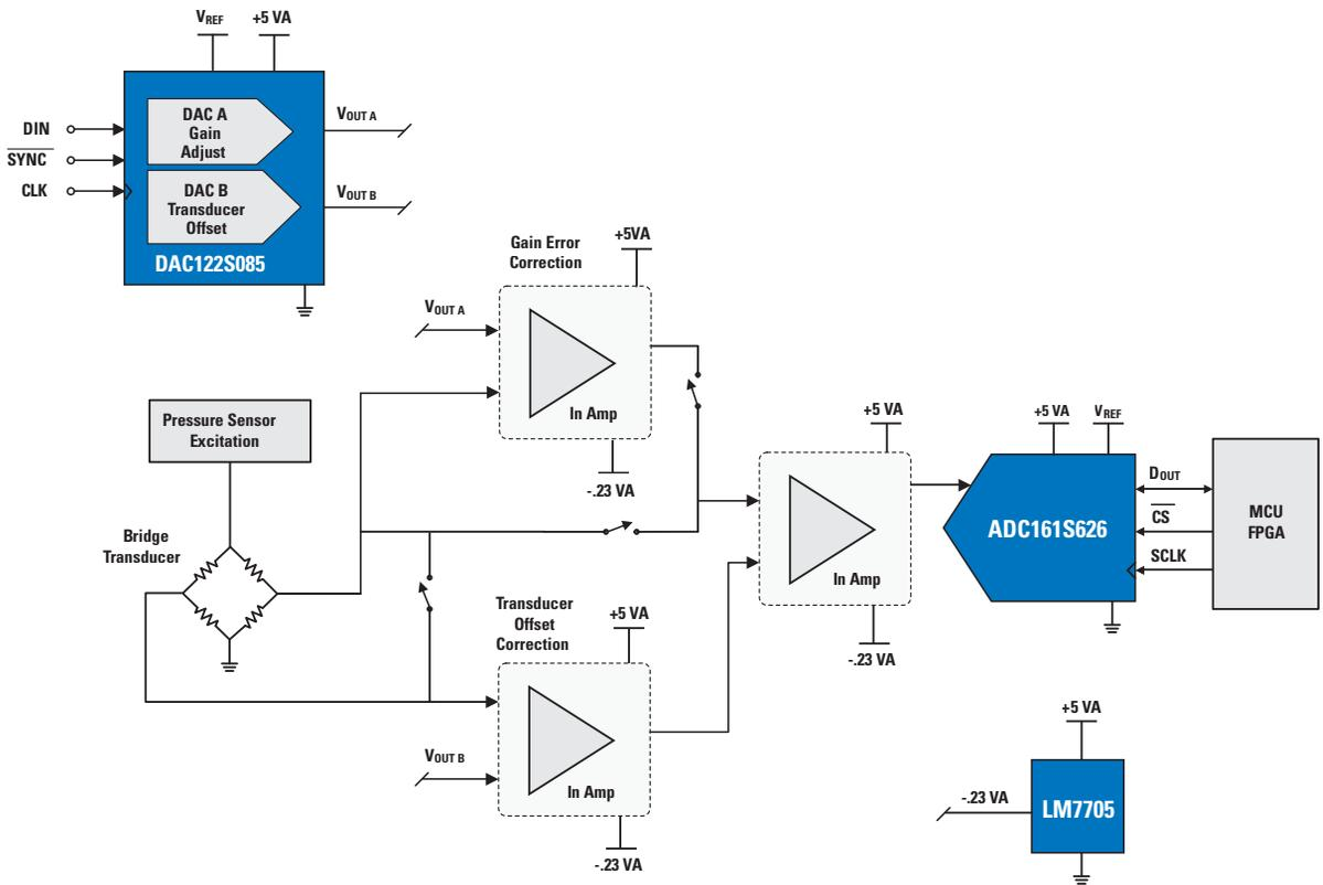
**Figure 2. Simplified Example of a Calibrated Pressure Sensing Diagram**
