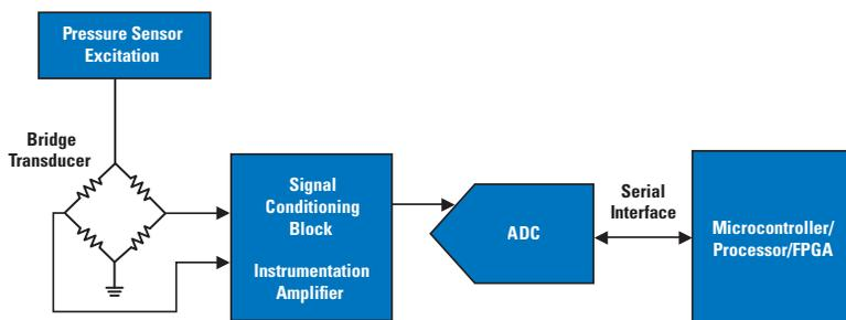
Figure 1. Pressure Sensing System Diagram
