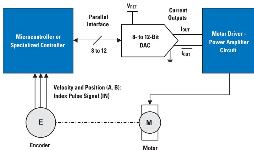
Figure 3. Motor Control Example
