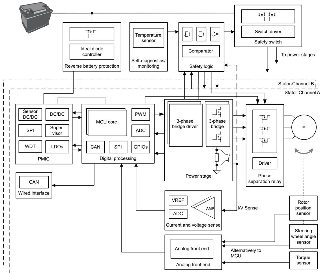
Figure 2. EPS System Block Diagram
