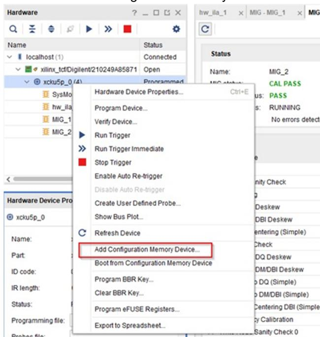
**Figure 3-1. Add Configuration Memory Device**
