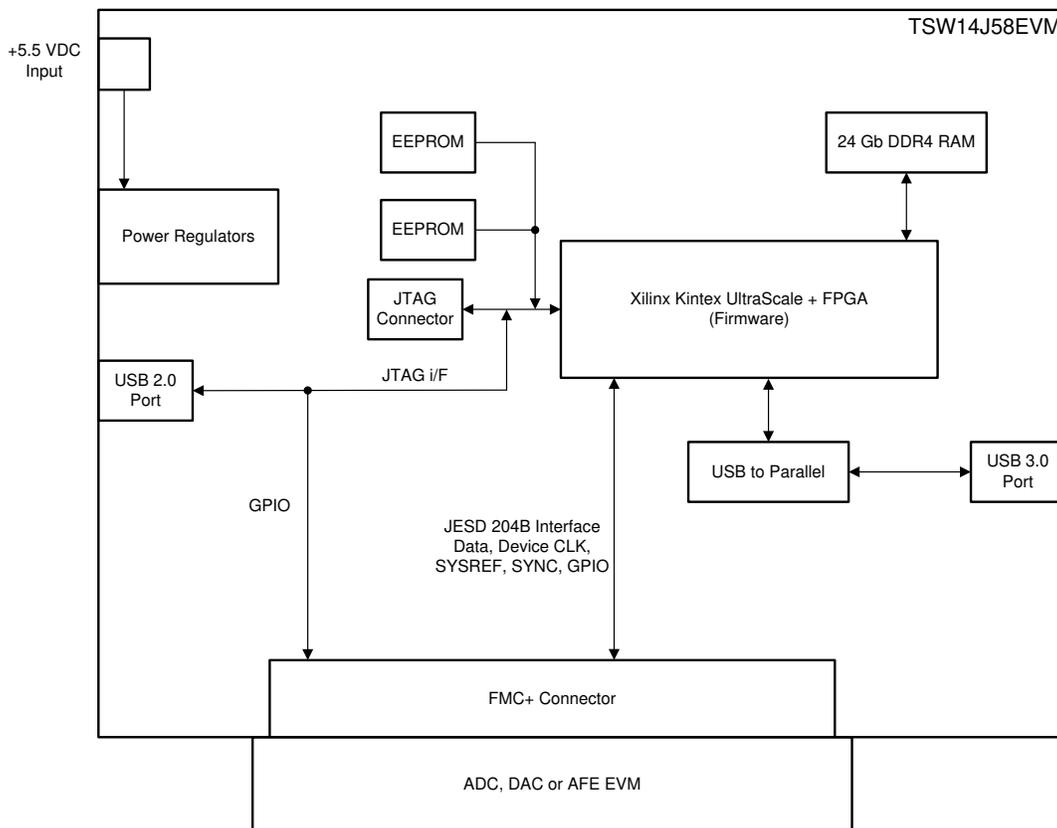
**Figure 2-2. TSW14J58EVM Block Diagram**
