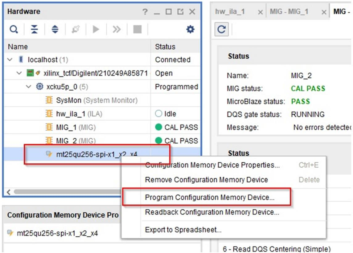
**Figure 3-2. Programming Memory Device**
