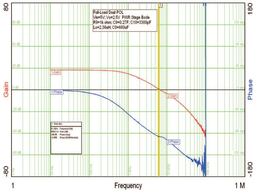
Figure 9. TPS50601SPEVM Power Stage Dual Mode
