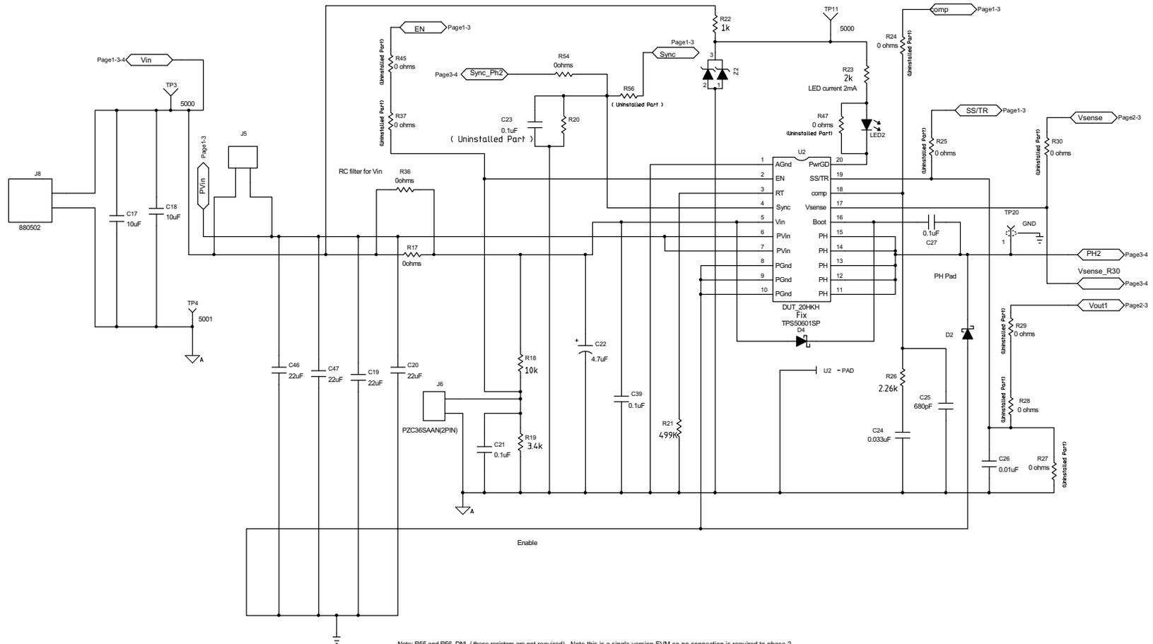
Note: R55 and R56 DNL ( these resistors are not required). Note this is a single version EVM so no connection is required to phase 2.
