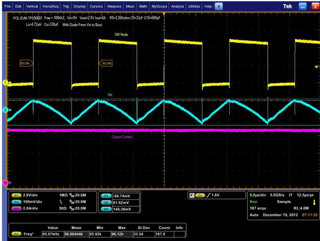
Figure 11. TPS50601SPEVM Input Ripple
