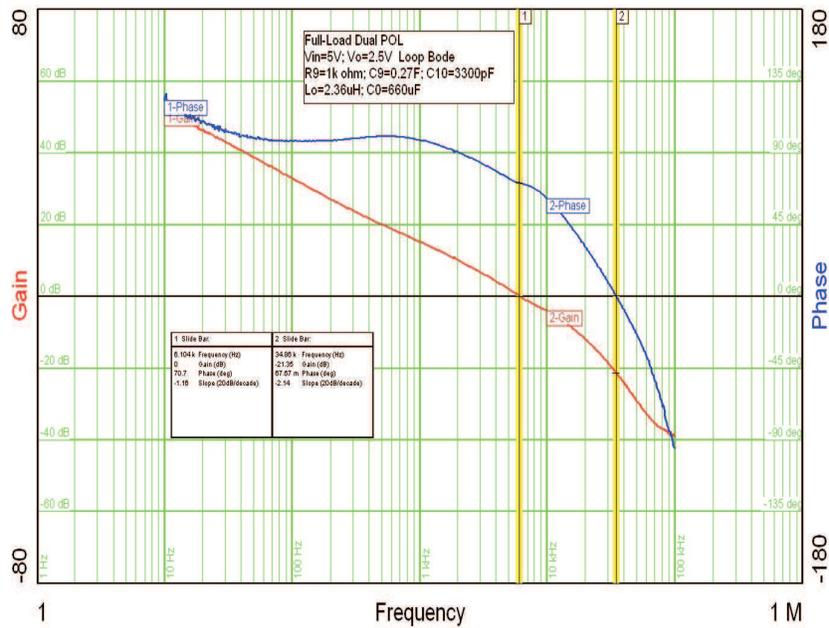
Figure 8. TPS50601SPEVM Loop Response Dual Mode
