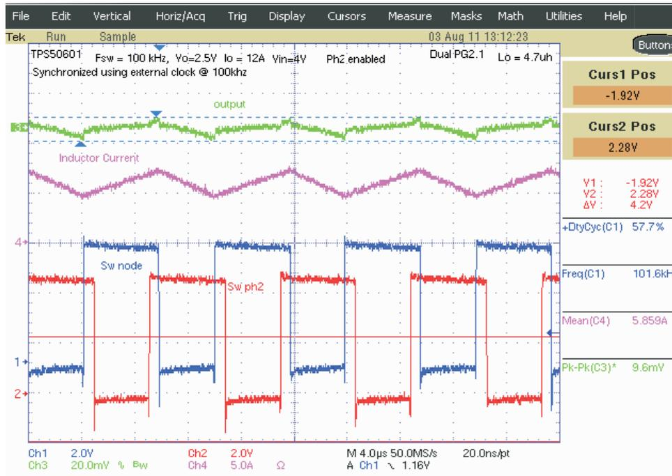
**Figure 12. Dual Phase Waveform**
