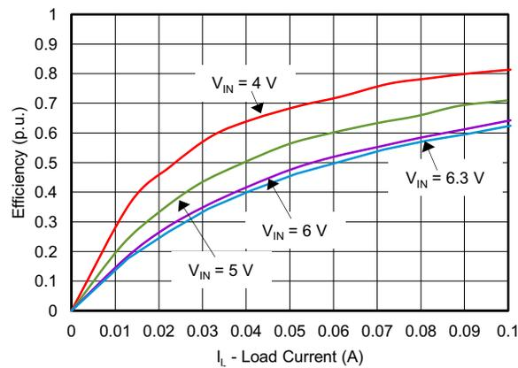
Figure 2. TPS50601SPEVM Low-Current Efficiency
