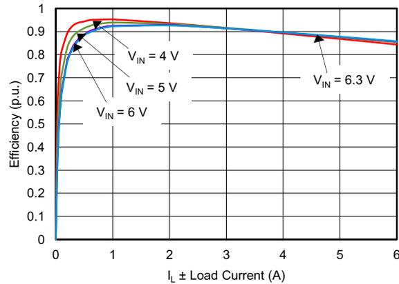
Figure 1. TPS50601SPEVM Efficiency
