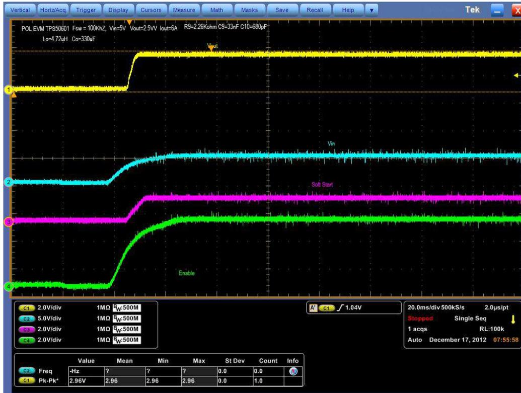
Figure 14. TPS50601SPEVM Start-Up Relative to V<sub>IN</sub>
