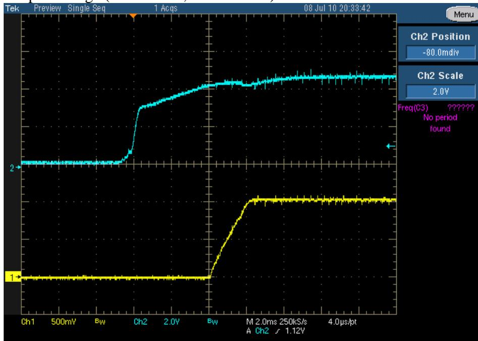
Startup behavior of the CORE, IO, DDR2 voltages after supplying the last input voltage (all the input voltages must be inside the nominal values before enabling any converter): the ENABLE\_NEG line goes down, thus enabling all converters.
