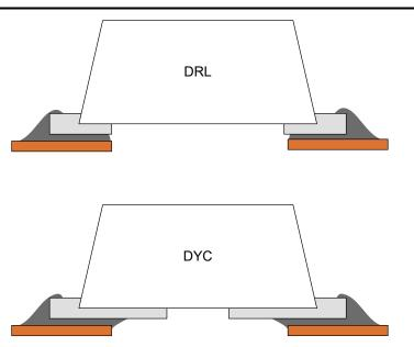
Figure 3. Cross-Section Illustration of Solder Distribution on DRL and DYC Packages
