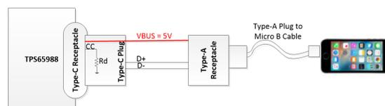
**Figure 2. USB Device Connection Via Type-A to Type-C adapter**
