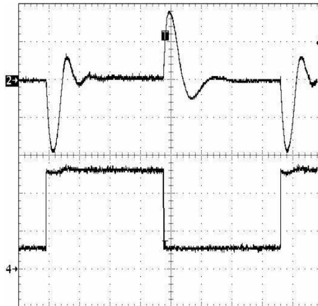
Figure 4. Undercompensated  $\rightarrow R_C$  is Too Small
