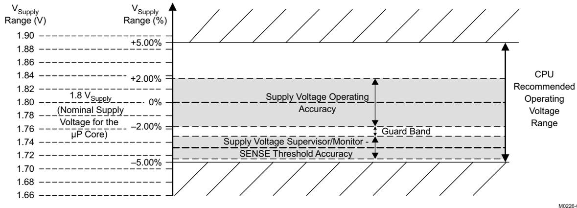
Figure 4. Illustration of a Nominal 1.8-V Power Supply, the Relative SVS Reset Threshold, and the Respective Accuracy Windows Necessary To Meet A “ $\pm 5\%$ ” CPU Operating Range Requirement
