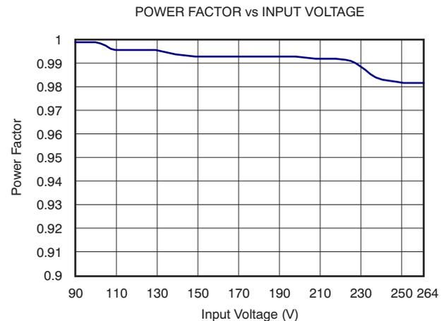
Figure 13. Power Factor at Full Load for PMP4298A
