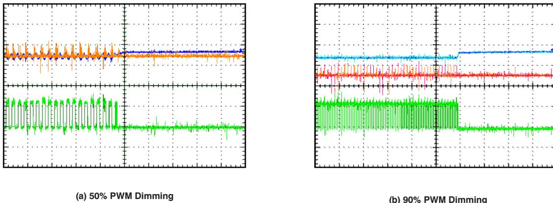
Figure 14. Output Headroom Voltage Waveforms for PMP4298A: LED ON to OFF
