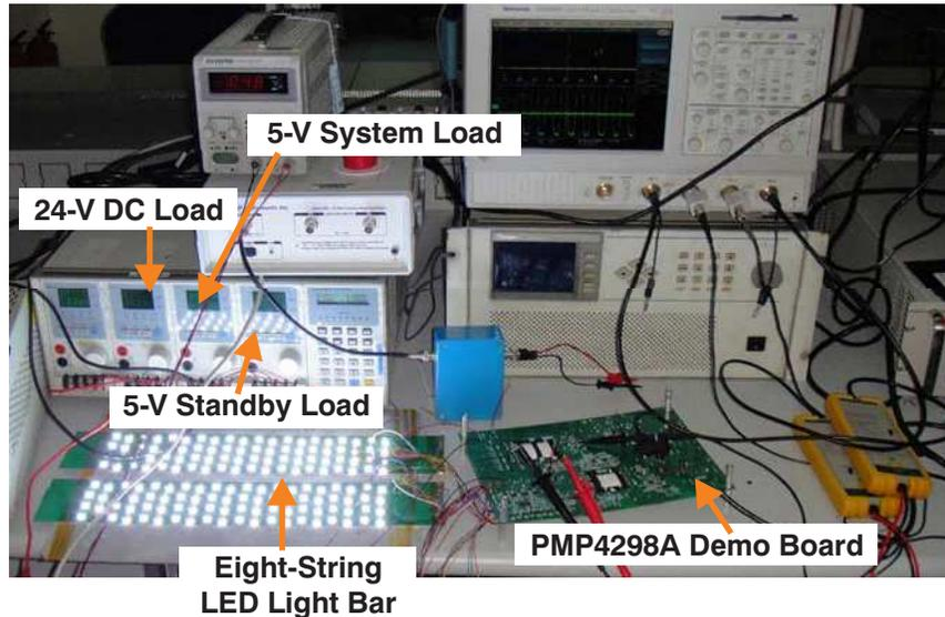
Figure 11. PMP4298A Demonstration Fixture Test Setup
