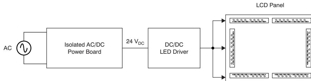
**Figure 1. Edge-Type LED Backlight LCD TV Power Conversion Scheme**
