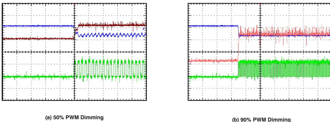
Figure 15. Output Headroom Voltage Waveforms for PMP4298A: LED OFF to ON
