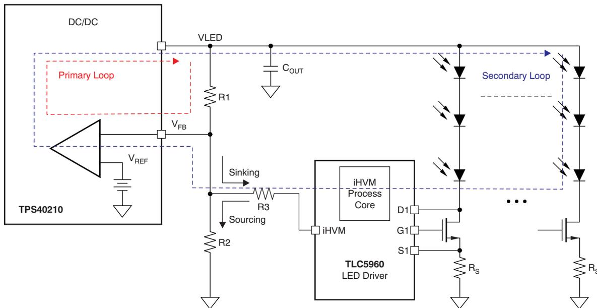
**Figure 4. PMP4298: iHVM Feedback Loop Integration into DC-DC Primary Feedback Loop**
