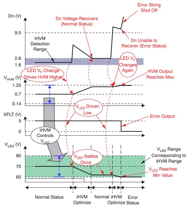
Figure 10. LED Short Detection and  $V_{LED}$  Optimization Through iHVM
