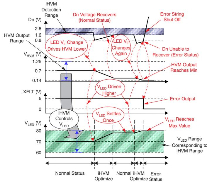
Figure 9. LED Open Detection and  $V_{LED}$  Optimization Through iHVM
