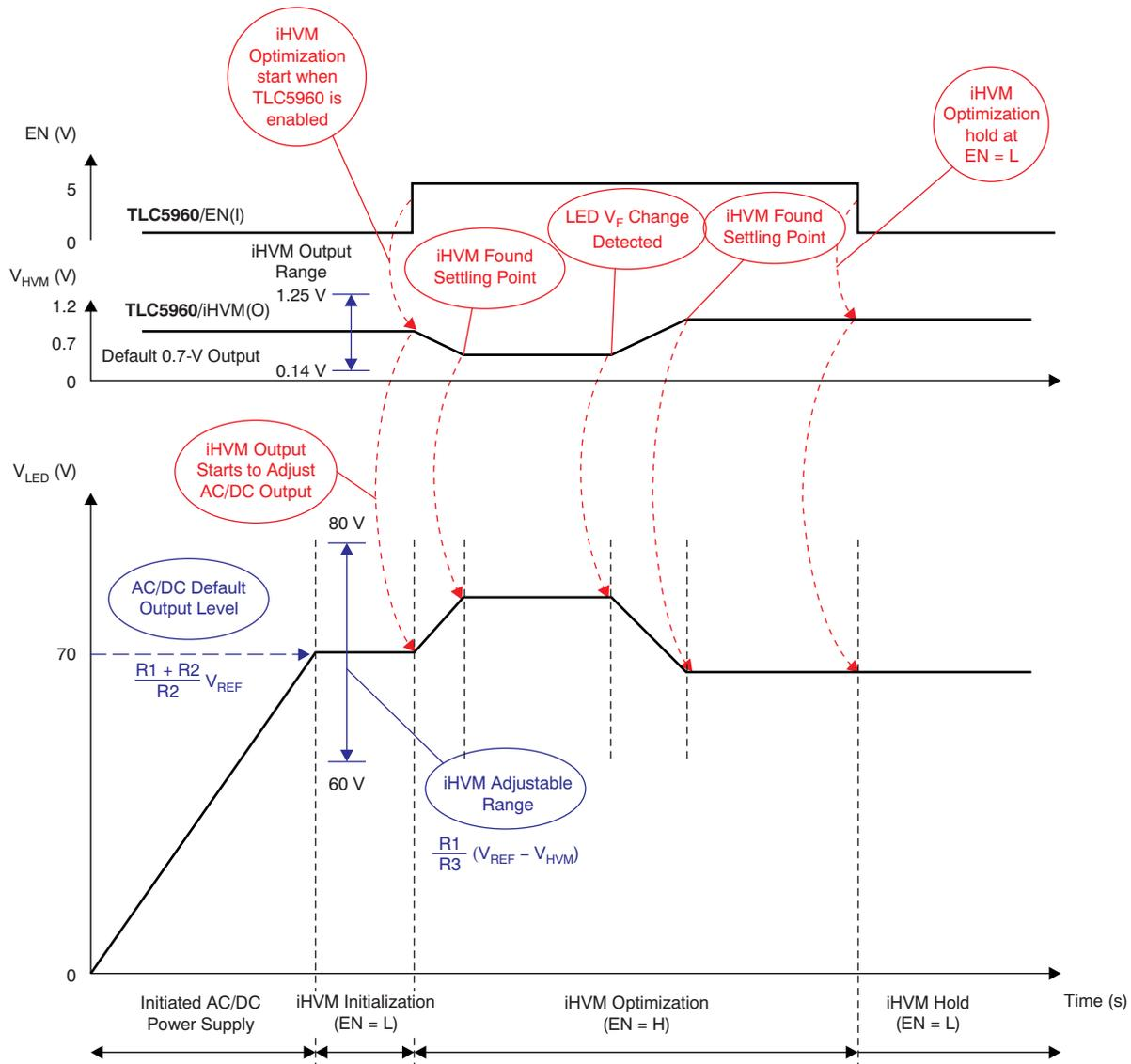
Figure 7. PMP4298A: AC-DC Power Stage Startup and iHVM Optimization Sequence
