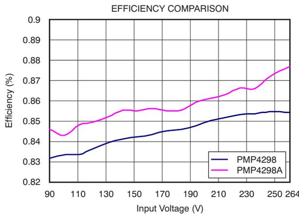
Figure 12. Total Efficiency Comparison at Full Load on V<sub>LED</sub>, 24 V and 5 V
