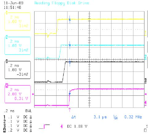
Figure 3. Sequencing in Start-Up Waveform
