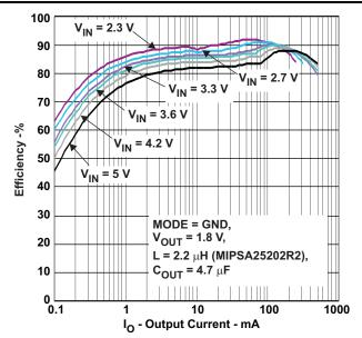
Figure 6. Efficiency vs Output Current
