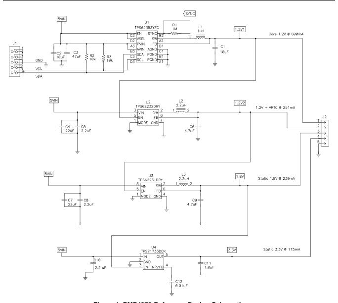
Figure 1. PMP4979 Reference Design Schematic
